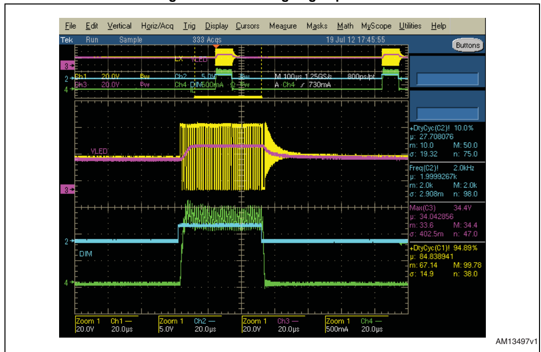
Figure 14. LED rising edge operation (zoom)
