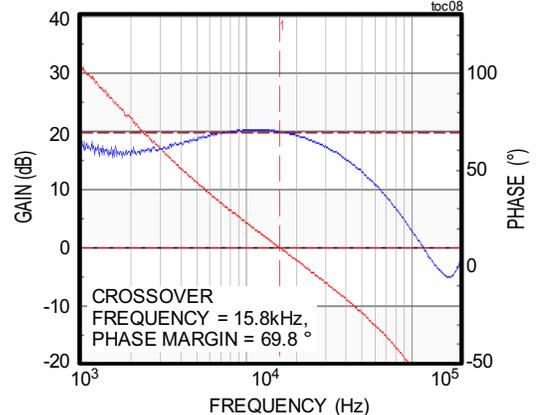
CONDITIONS:  $f_{SW} = 400\text{kHz}$ , 24V INPUT
