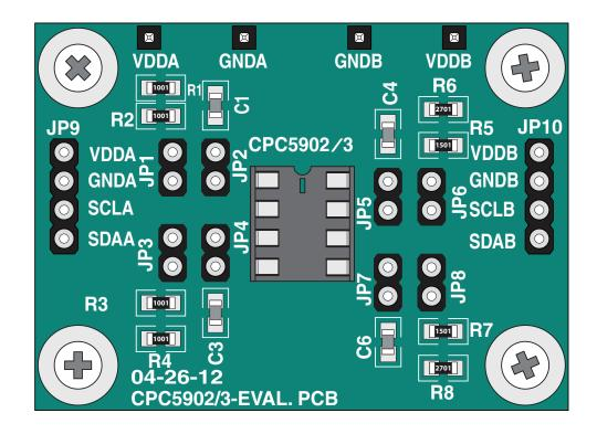
The CPC5902G/5903G Evaluation Board can be used to isolate an I<sup>2</sup>C bus, and to evaluate the performance obtainable when communicating between the user's I<sup>2</sup>C devices. The 8-pin DIP socket can be populated with either a CPC5902G (for both SCL and SDA bidirectional) or with a CPC5903G (for SDA bidirectional, SCL sideA to sideB only).
