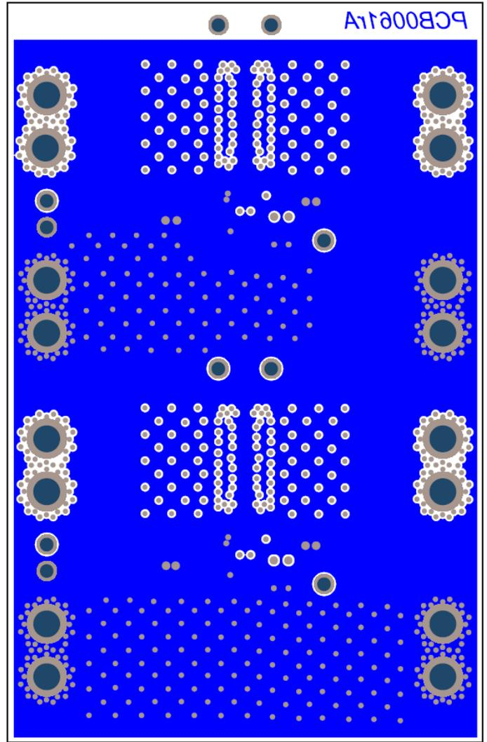
Figure 9: PI5101-EVAL1 layout bottom layer 2. Scale 2.0:1
