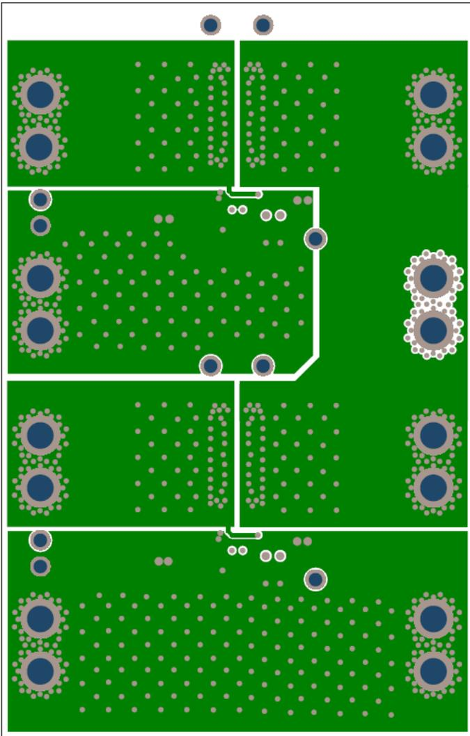
Figure 8: PI5101-EVAL1 layout mid layer 1. Scale 2.0:1
