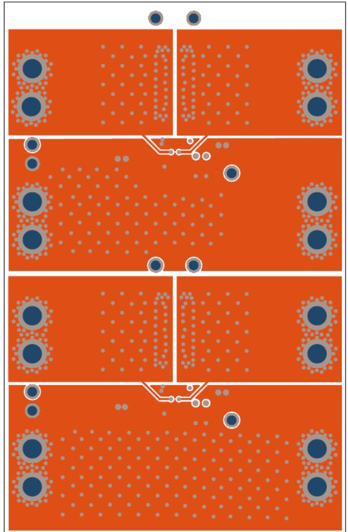
Figure 7: PI5101-EVAL1 layout mid layer 2. Scale 2.0:1
