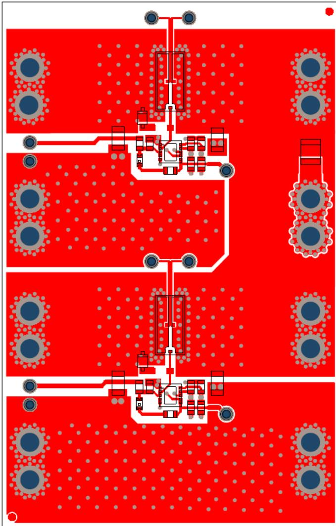
Figure 6: PI5101-EVAL1 layout top layer. Scale 2.0:1
