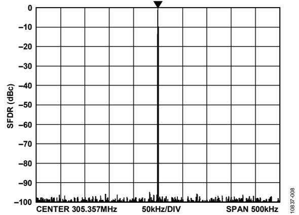
Figure 8. Narrow-Band SFDR at 305.3 MHz,
