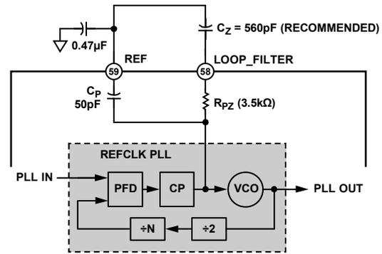
Figure 34. REF CLK PLL External Loop Filter
