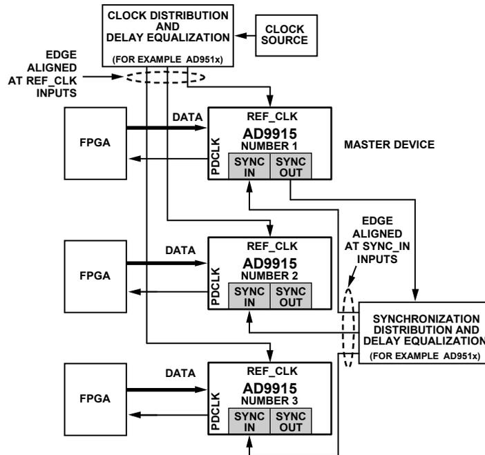
Figure 49. Configuration of Multiple Devices to Be Synchronized
