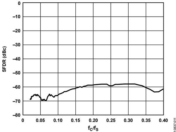
Figure 11. Wideband SFDR vs. Normalized  $f_{OUT}$ , SYSCLK = 2.5 GHz
