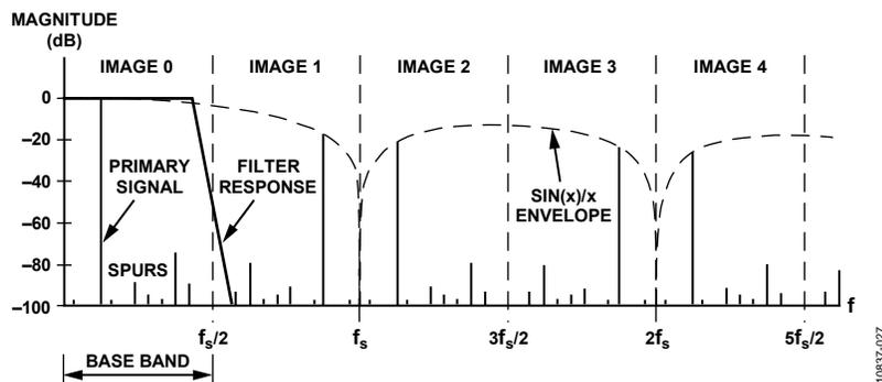
Figure 31. DAC Spectrum vs. Reconstruction Filter Response
