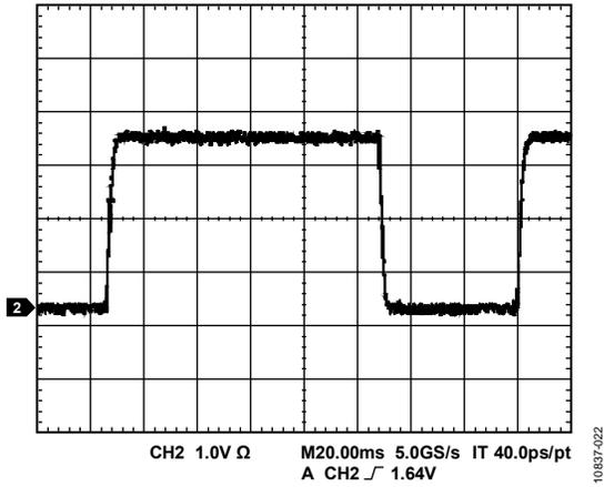
Figure 22. SYNC\_OUT ( $f_{SYSCLK}/384$ )
