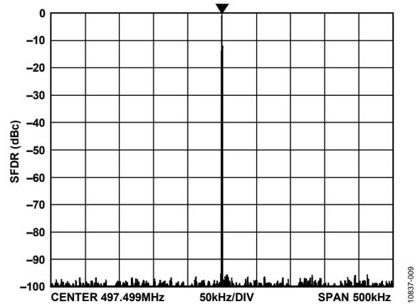
Figure 9. Narrow-Band SFDR at 497.5 MHz,
