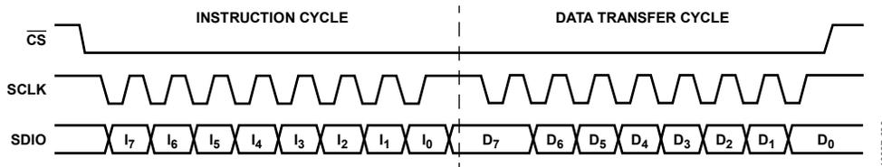
Figure 44. Serial Port Write Timing, Clock Stall High
