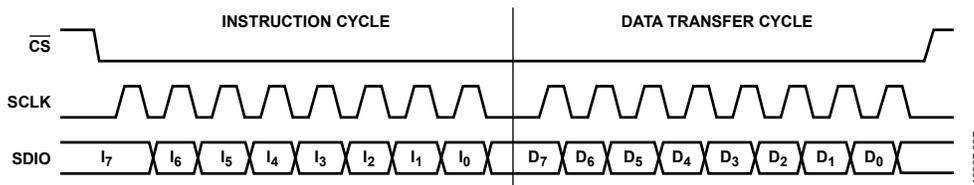
Figure 42. Serial Port Write Timing, Clock Stall Low
