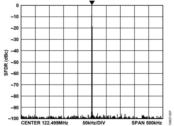
Figure 7. Narrow-Band SFDR at 122.5 MHz,
