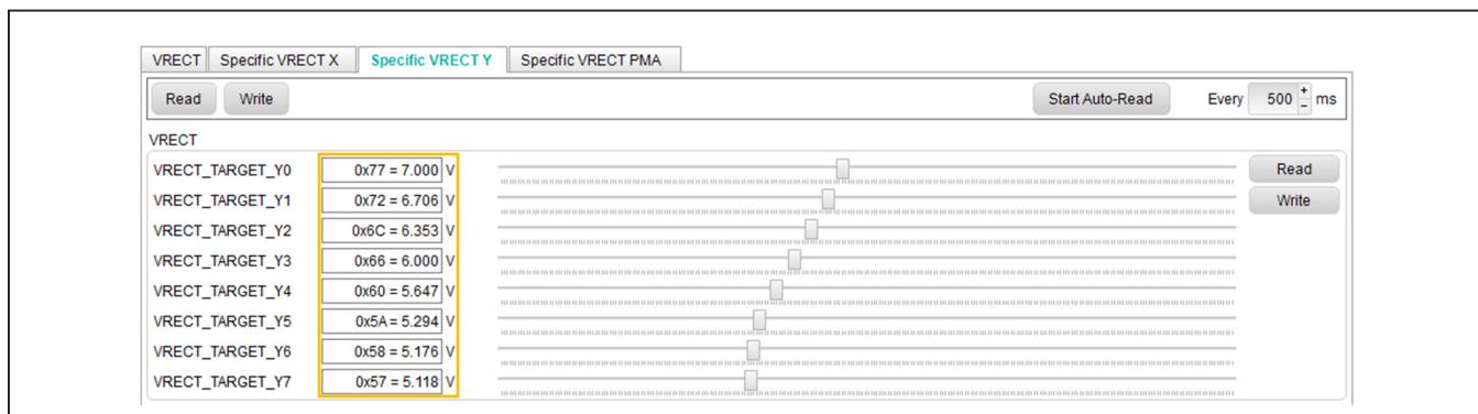
Figure 6. MAX77950 EV Kit GUI (VRECT-RX Tab)
