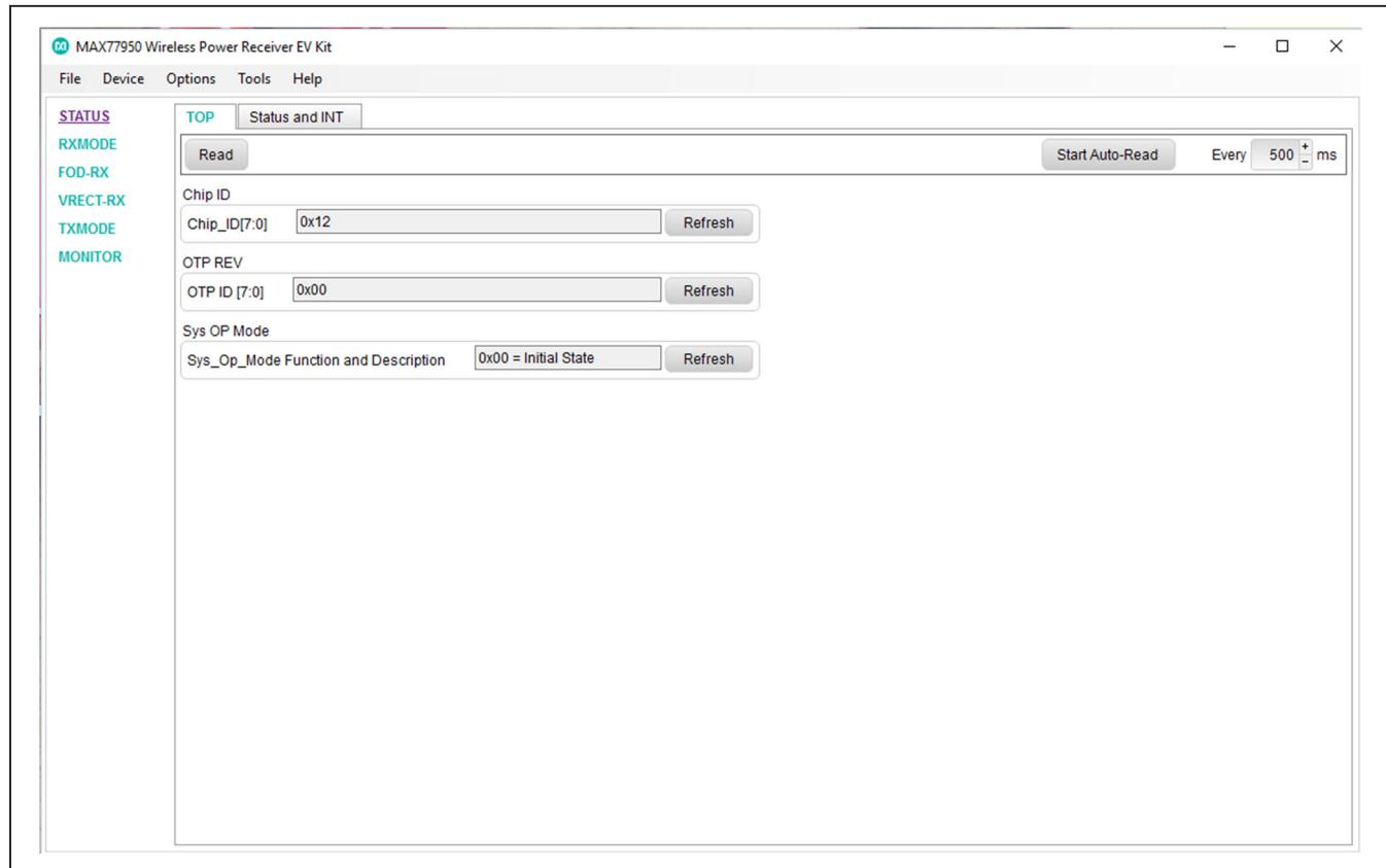
Figure 2. MAX77950 EV Kit GUI (STATUS Tab)
