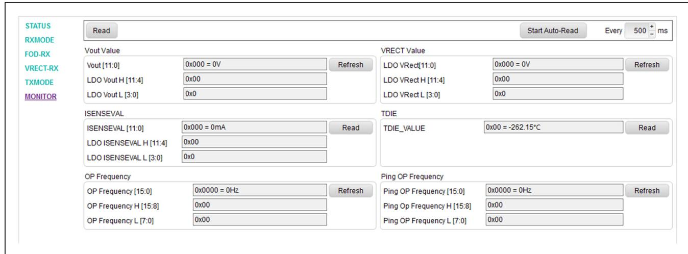
Figure 8. MAX77950 EV Kit GUI (MONITOR Tab)
