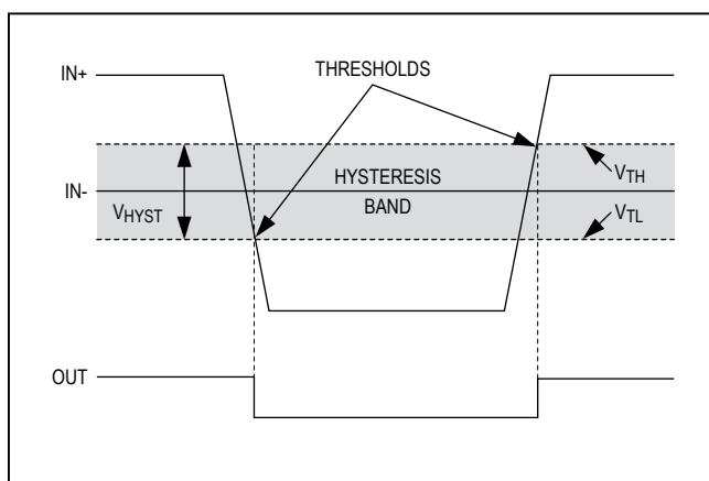
Figure 1. Threshold Hysteresis Band (Not to Scale)
