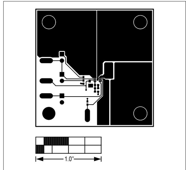
Figure 3. MAX15062C 12V EV Kit PCB Layout—Component Side
