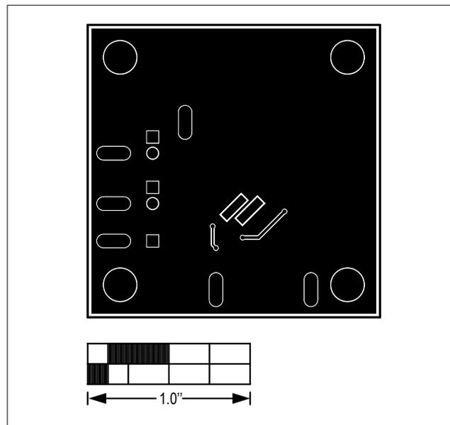
Figure 4. MAX15062C 12V EV Kit PCB Layout—Solder Side
