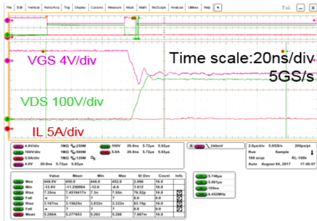
Figure 16(b): Typical turn-off waveform
