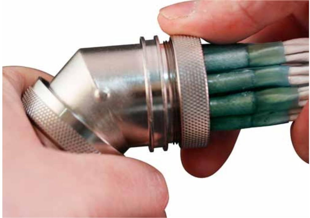
Tighten the gland nut on the body to the appropriate torque value.
