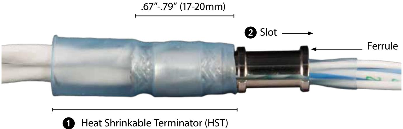
2 Next, carefully slide the StarShield™ ferrule (with slotted side oriented towards contacts) over the leads until the non-lipped end slides under the HST braid. Cable jacketing should be positioned on the ferrule as shown above.
