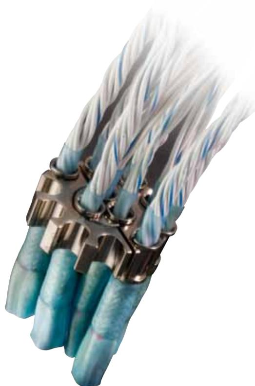
Position the sub-assemblies (stars, compression ring and ferrules) into the body by carefully twisting to “birdcage” the individual wire pairs first and then the entire wire bundle in a counter clockwise motion. If necessary, heat may be applied to the wires to make them more pliable and easier to fit into backshell body (Hot air gun setting 4–5 or 450°–520°F/230°–270°C with reducer nozzle).
