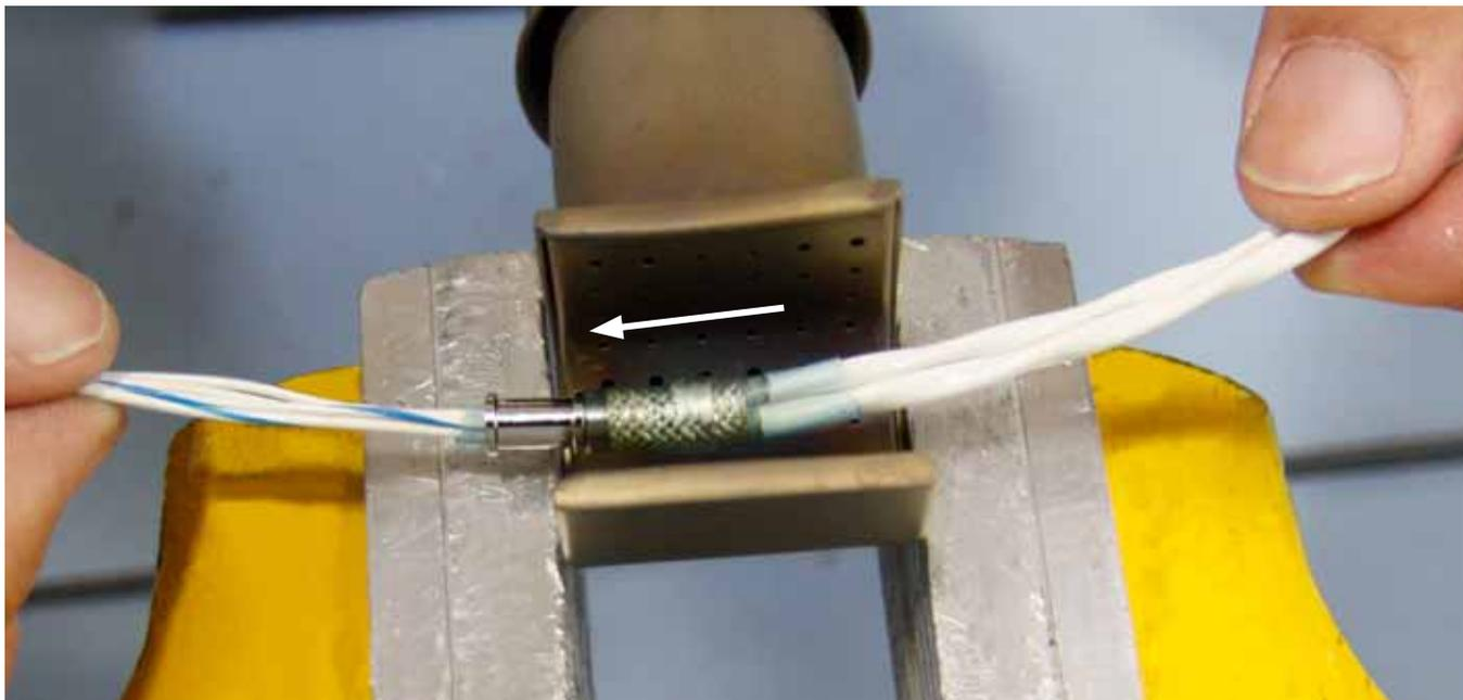
Focus heat on ferrule for a few seconds and begin moving towards the solder preform. Solder should melt and begin to flow freely. Continue to move the preform towards the center of the heat reflector as solder completely melts and flows along preform braid.
