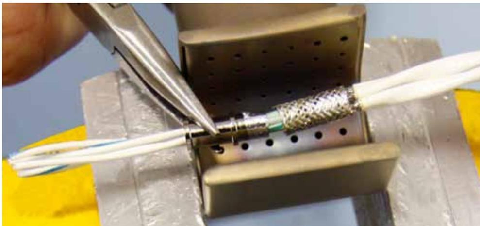
Next, grasp preform braid with needle nose pliers and return assembly to hot air gun reflector. When solder begins to melt, gently pull preform braid away from cable. Remove from heat and allow to cool.
