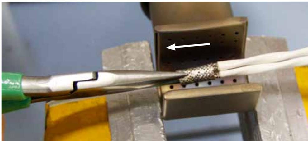
Once assembly cools to ambient temperature, use fingers to gently scrape residual solder off cable jacketing and protective sleeve.
