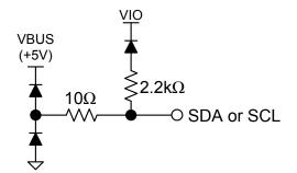
VIO is the programmed Target I/O voltage of the Adapter. The GP3/VDD pin has the following equivalent input circuit, assuming the pin is operating as GP3:
