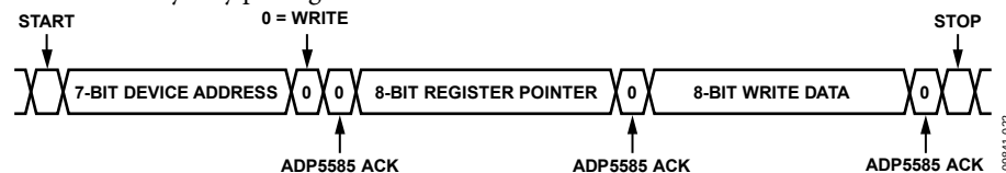
Figure 23. I 2 C Single Byte Write Sequence
