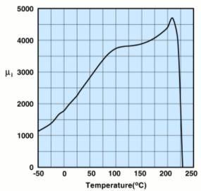
Measured on an 18/10/6mm toroid at 100kHz.
