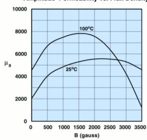
Measured on an 18/10/6mm toroid at 10kHz.
