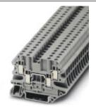
Four-conductor universal terminal block, Connection method: Screw connection, Cross section: 0.14 mm² - 6 mm², AWG: 26 - 10, Width: 6.2 mm, Color: red, Mounting type: NS 35/7,5, NS 35/15
