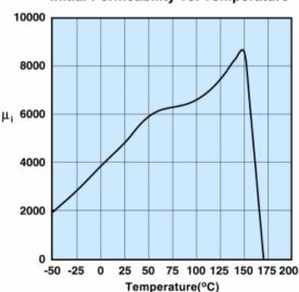
Measured on a 17/10/6mm toroid at 10kHz.
