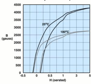
Measured on a 17/10/6mm toroid at 10kHz.
