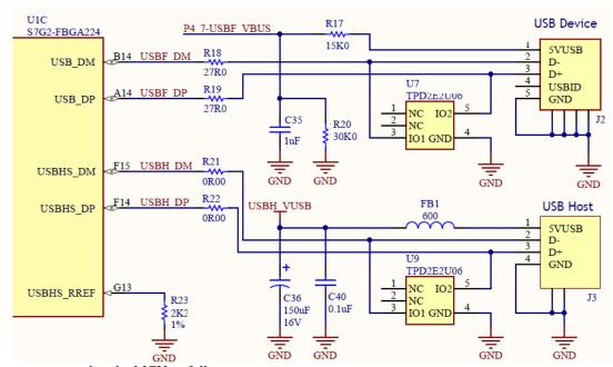
The ports are connected to the MCU as follows:
