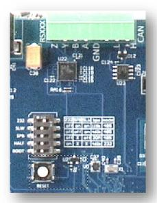
The large green 3.5-mm connector J10 delivers RS232, RS422, or RS485 as well as high performance CAN to external industrial networks. A screw terminal plug is supplied, enabling easy wiring of termination or daisy chained cabling. The connector's signals are clearly marked on the PCB as follows:
