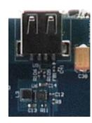
**R13** sets the current limit: in this design  $51.0k\Omega$  indicates a limit of ~500mA. At currents above this limit, the voltage on the output to the connector drops precipitously to limit the current to this maximum. The **FAULT#** open drain output from the chip indicates when the chip is in current-limiting mode and can be used by software to detect this fault condition.
