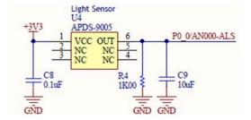
3.3 V on an Analog to Digital Converter (ADC) input on the MCU. Software can poll this ADC periodically. The ALS is connected as follows:
