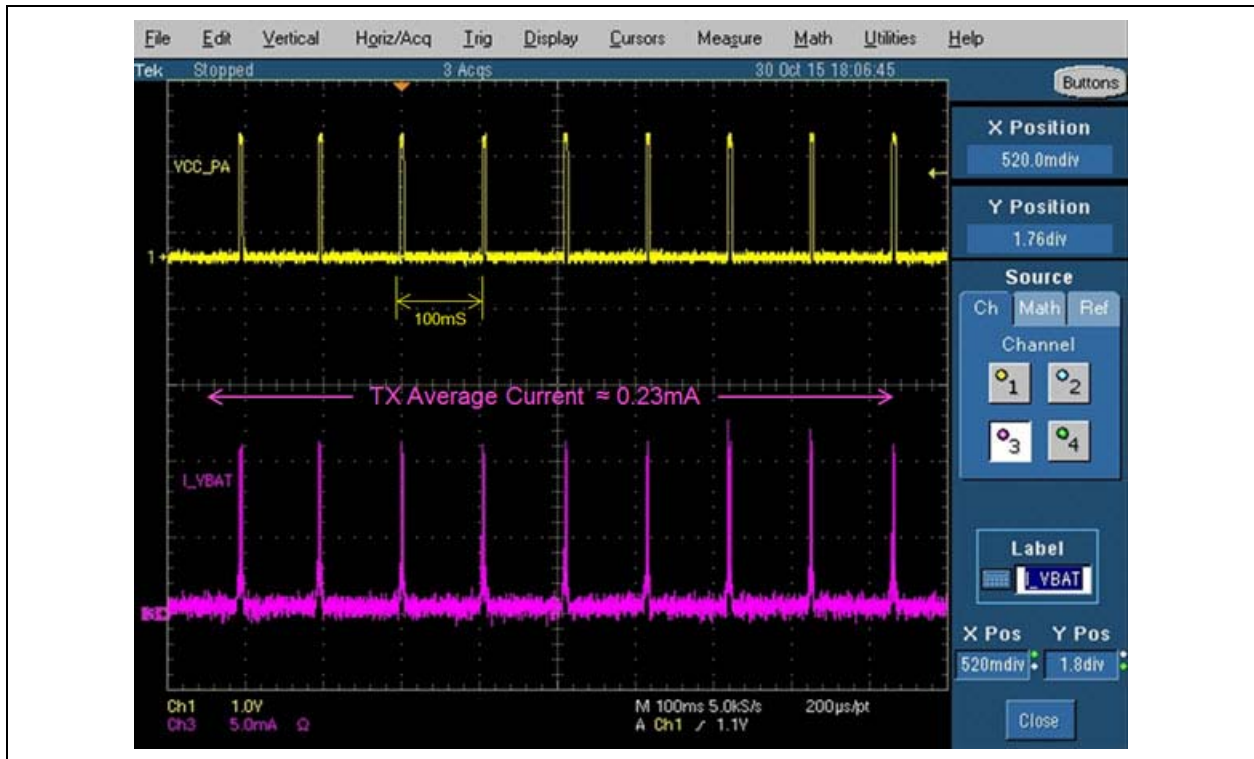
FIGURE 5-2: TX/RX AVERAGE CURRENT CONSUMPTION WHILE BM70/71 MODULE IS ADVERTISING
