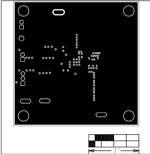
Figure 4. MAXM17504 EV Kit PCB Layout—PGND Layer 2
