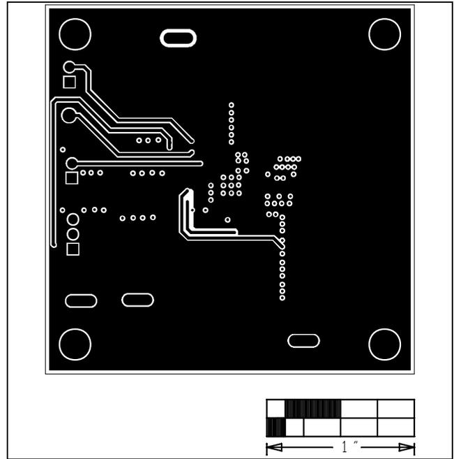
Figure 5. MAXM17504 EV Kit PCB Layout—PGND Layer 3
