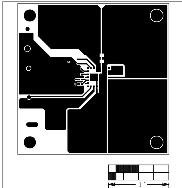
Figure 3. MAXM17504 EV Kit PCB Layout—Component Side
