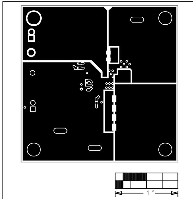
Figure 6. MAXM17504 EV Kit PCB Layout—Solder Side
