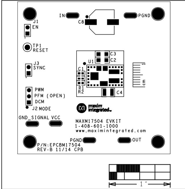
Figure 1. MAXM17504 EV Kit Component Placement Guide—Component Side
