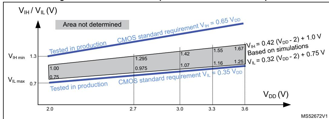
**Figure 23. 5 V tolerant I/O input characteristics - TTL port**
