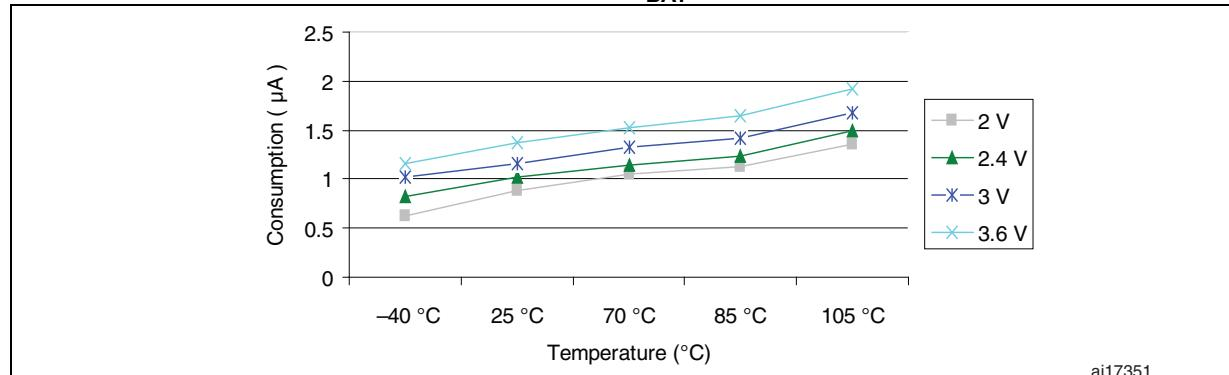
**Figure 13. Typical current consumption in Stop mode with regulator in Run mode versus temperature,  $V_{DD} = 3.3 / 3.6 \text{ V}$**
