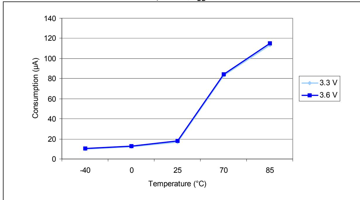
**Figure 15. Typical current consumption in Standby mode versus temperature,  $V_{DD} = 3.3 / 3.6 \text{ V}$**
