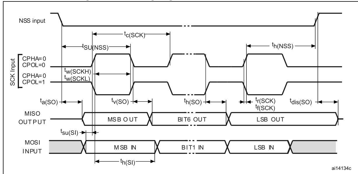
Figure 28. SPI timing diagram - slave mode and CPHA=1<sup>(1)</sup>
