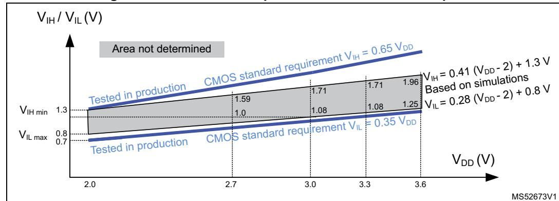
**Figure 21. Standard I/O input characteristics - TTL port**
