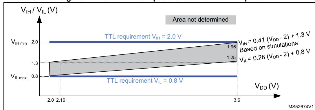
**Figure 22. 5 V tolerant I/O input characteristics - CMOS port**
