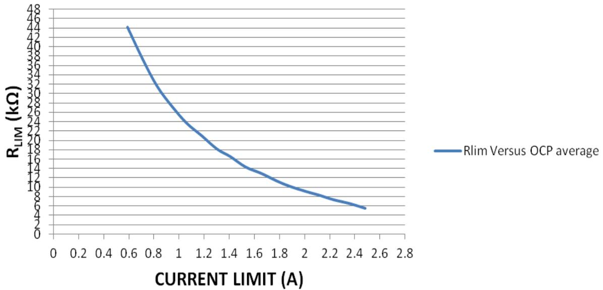
Figure 25. R<sub>lim</sub> Curve versus Current Limit
