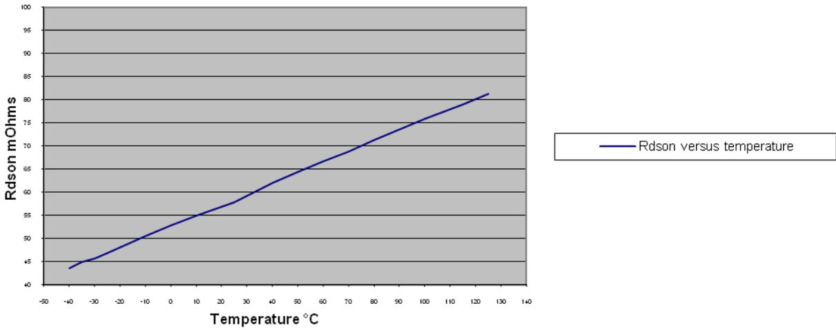
Figure 21. R<sub>DS(on)</sub> vs Temperature, μDFN Package
