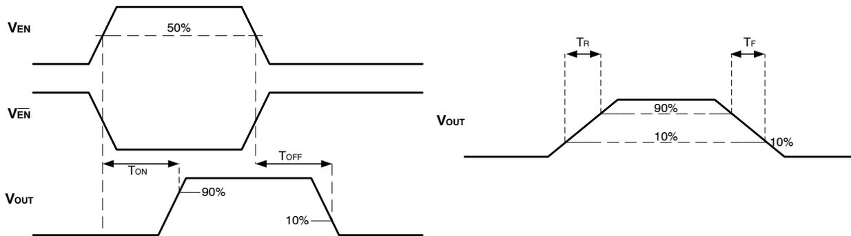
**Figure 4. Voltage Waveform**
