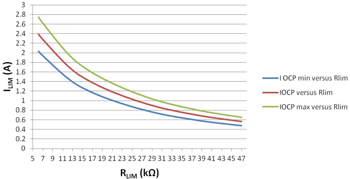
**Figure 26. Current Threshold vs R<sub>LIM</sub> Resistor**
