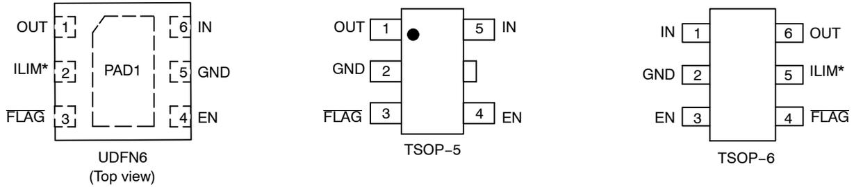
Figure 2. Pin Connections
