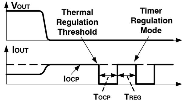
Figure 24. Short circuit
