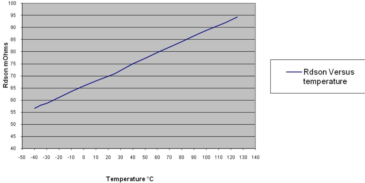
Figure 20. R<sub>DS(on)</sub> vs Temperature, TSOP Package
