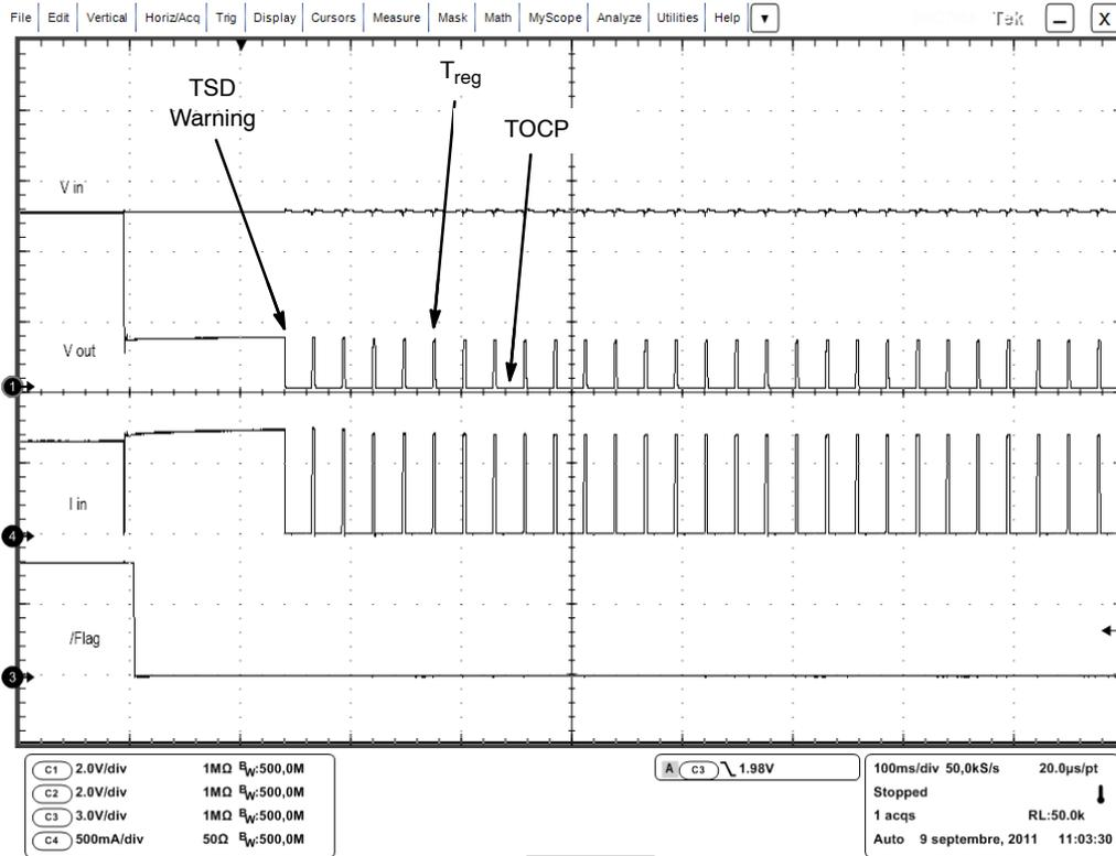
Figure 9. 2 Ω Short on Output. Complete Regulation Sequence
