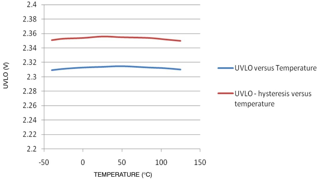
Figure 17. Undervoltage Threshold (Falling) and Hysteresis
