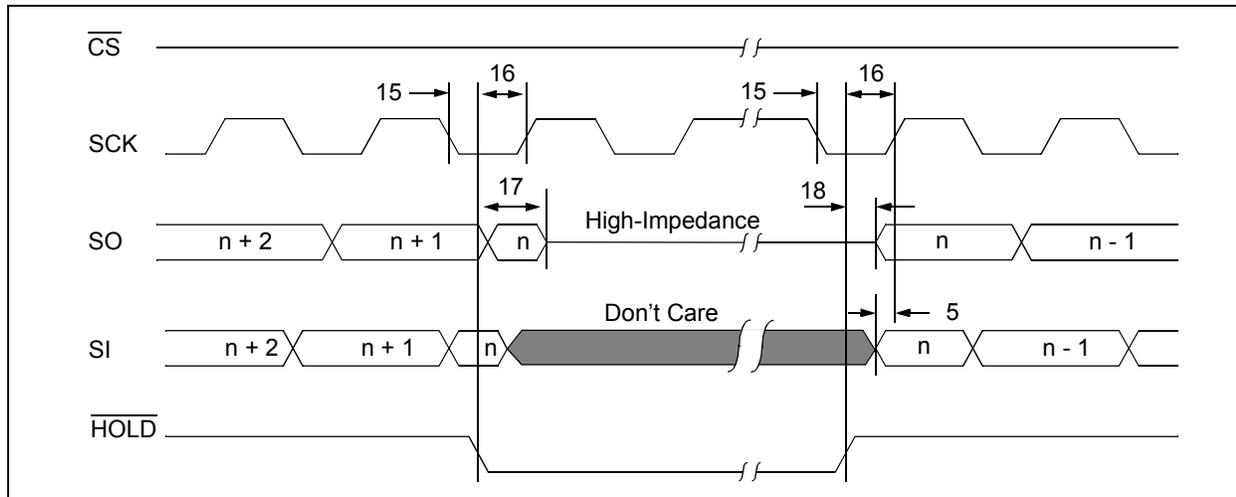
**FIGURE 1-2: SERIAL INPUT TIMING (SPI MODE)**
