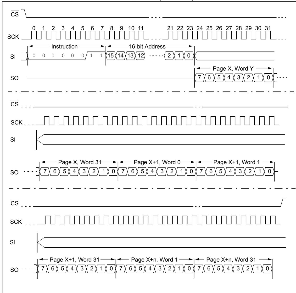
**FIGURE 2-6: SEQUENTIAL WRITE SEQUENCE (SPI MODE)**
