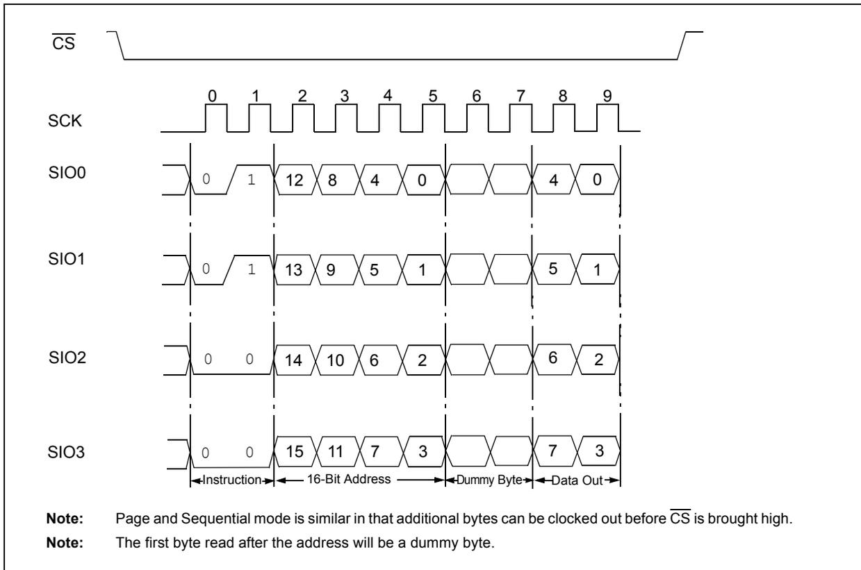
**FIGURE 4-6: BYTE WRITE MODE SQI**
