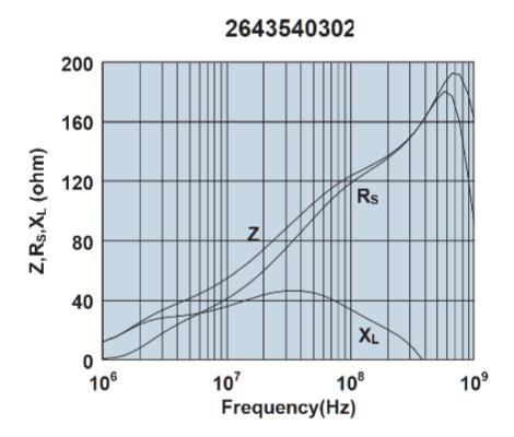
Impedance, reactance, and resistance vs. frequency.
