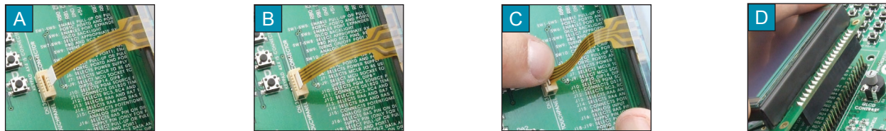
Figure 16-3: Connecting touch panel
