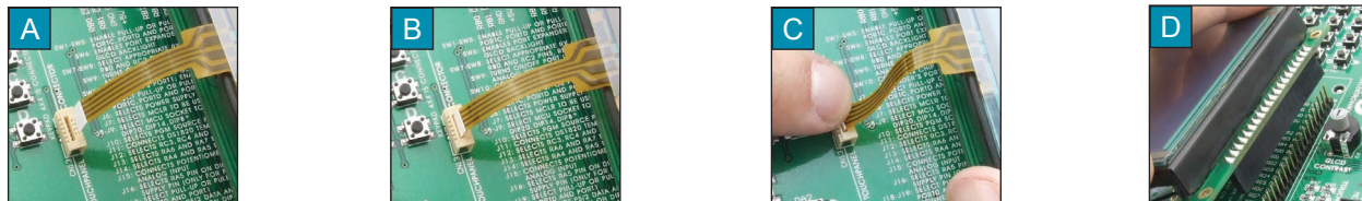
Figure 16-3: Connecting touch panel
