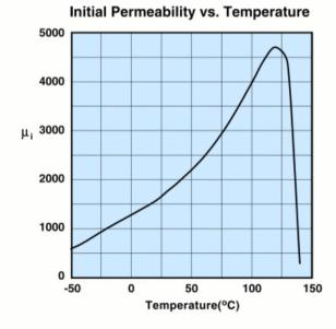
Measured on a 17/10/6mm toroid at 100kHz.
