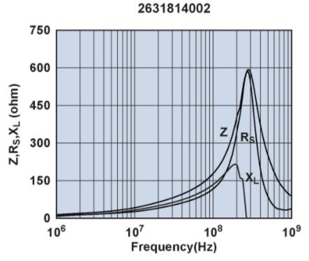
Impedance, reactance, and resistance vs. frequency.
