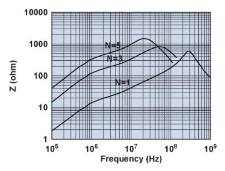
Impedance vs. frequency with one, three, and five turns.
