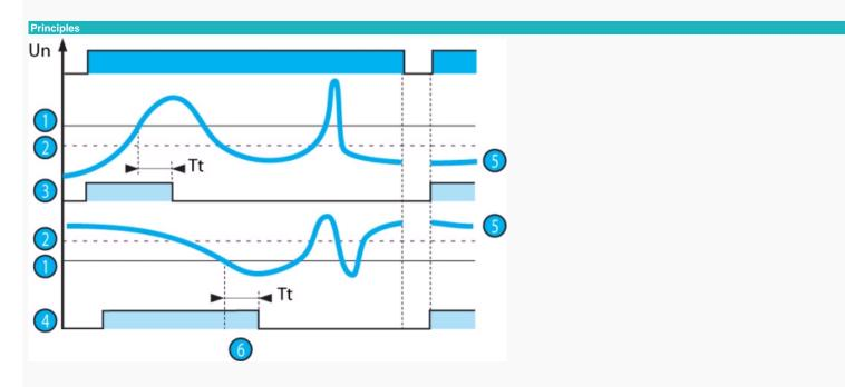
If "with memory" mode has been selected, the relay opens and stays in this position when threshold crossing is detected. The power supply must be disconnected to reset the product.
