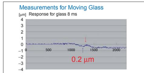
Ideal for measuring glass thickness and slit nozzle gaps when coating glass with resist or sealer.
