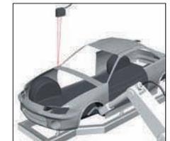
Protruding objects and steps can be measured from a distance for measurement objects that cannot be accessed easily.
