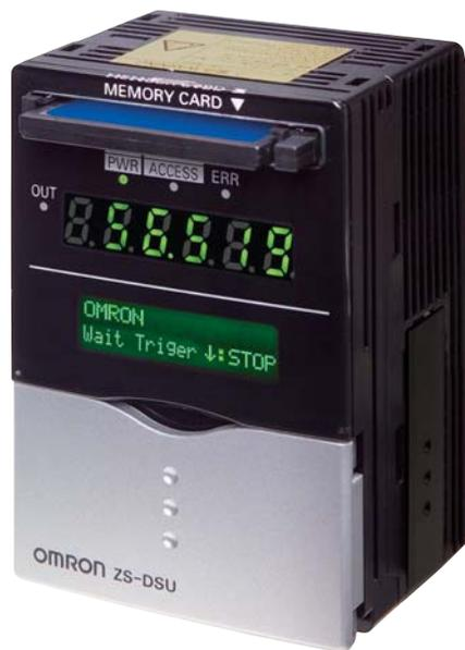
Efficiently stores sensing data using a variety of logging functions.
