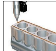
Ideal for measuring liquid gasket (FPIG) application amounts. Prevents defects such as insufficient seal.
