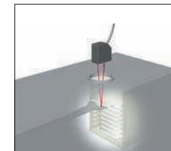
Ideal for checking the flatness of robot arms that transport wafers in load ports.
