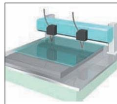
Ideal for measuring glass thickness and nozzle gaps when coating glass with resist or sealer.
