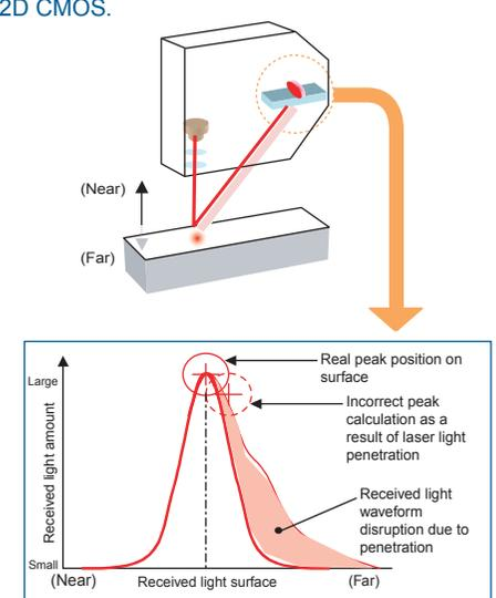
Real surface displacement detected by eliminating penetration effects for PCBs, plastic, and other workpieces penetrated by laser light.
