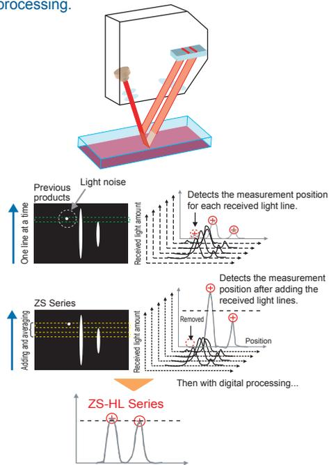
Measurement cycle time 1/8 better than previous models with addition of received light waveform captured by 2D CMOS and simultaneous measurement of front and back glass surfaces with separate sensitivities.
