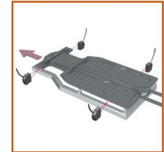
Manage trends by measuring widths of each car model.
