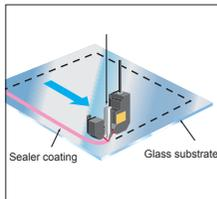
Ideal for measuring and controlling dispenser nozzle gaps when applying sealer.
