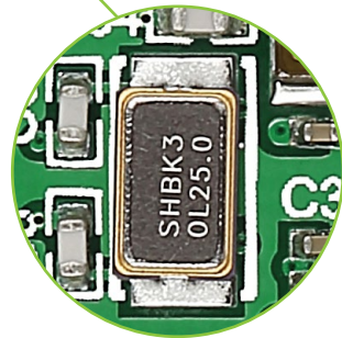
Figure 6-2: 25MHz crystal oscillator module (X1)
