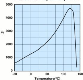
Measured on a 17/10/6mm toroid at 100kHz.
