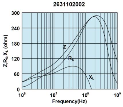
Impedance, reactance, and resistance vs. frequency.
