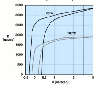
Measured on a 17/10/6mm toroid at 10kHz.
