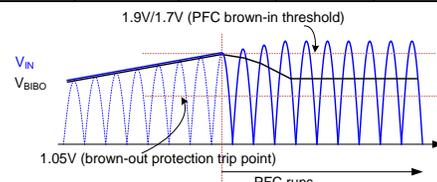
Figure 19.  $V_{BIBO}$  According to the PFC Operation
