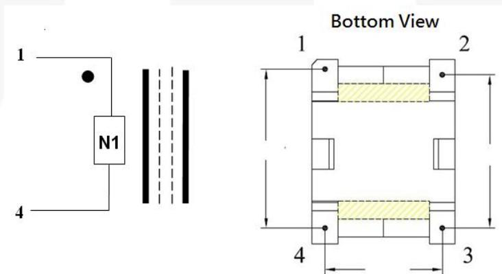
Figure 53. Inductor Schematic Diagram
