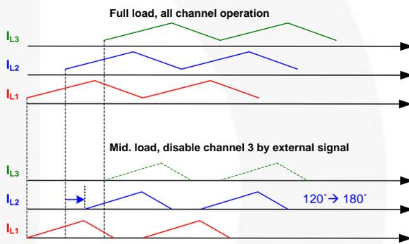
Figure 17. Phase Change under External Signal Control
