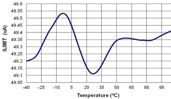
Figure 46.  $I_{LIMIT2}$  vs. Temperature
