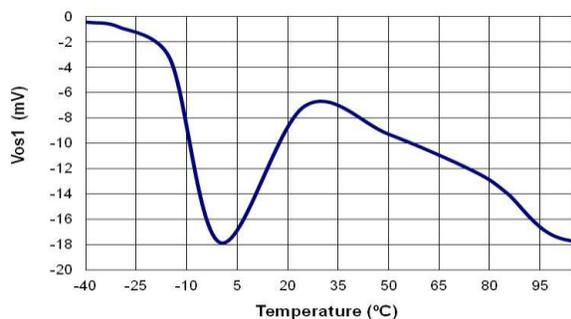
Figure 40.  $V_{OFFSET}$  vs. Temperature
