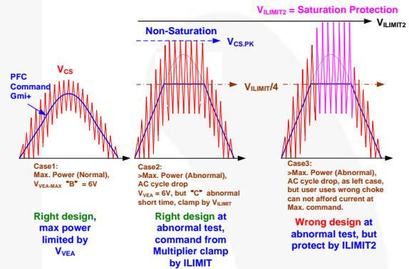
Figure 23. I<sub>LIMIT</sub> and I<sub>LIMIT2</sub> Setting
