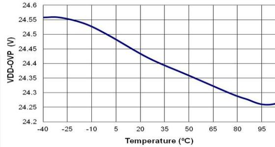
Figure 31.  $V_{DD-OVP}$  vs. Temperature
