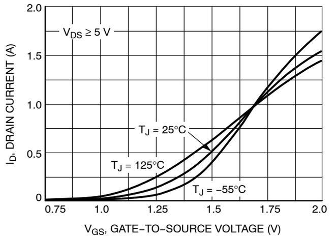
Figure 2. Transfer Characteristics
