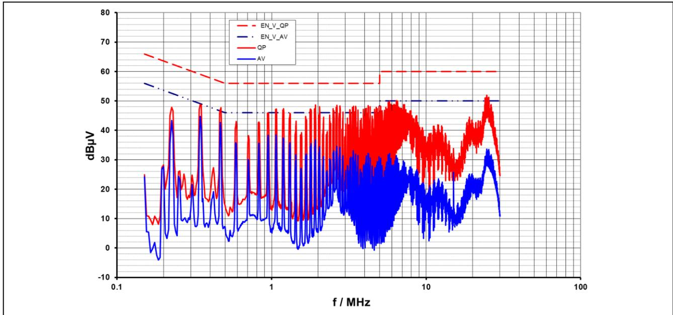
Figure 15 Conducted emissions(line) at 230 V<sub>AC</sub> and maximum Load
