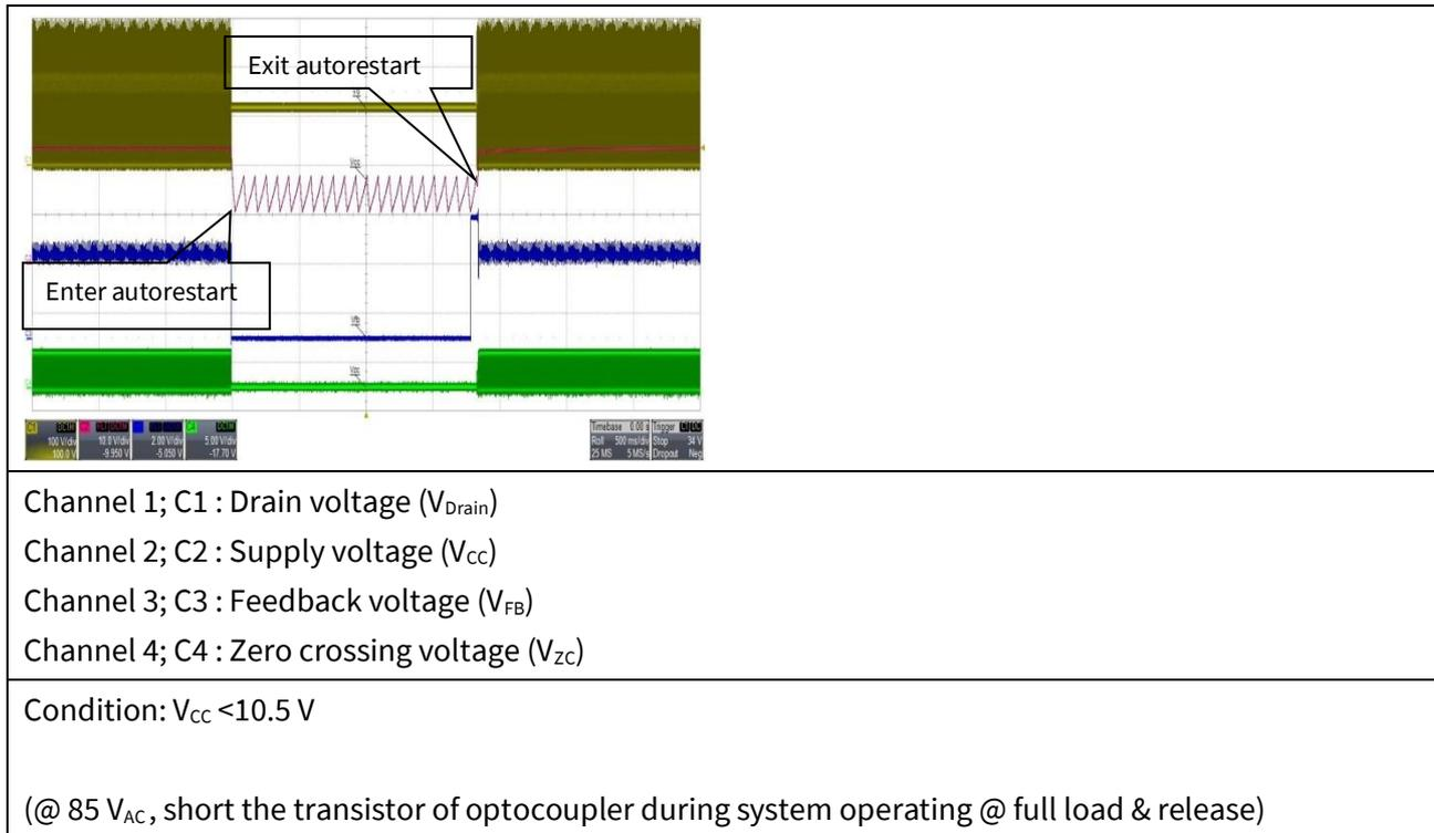
**Figure 30  $V_{CC}$  under voltage/short optocoupler protection**
