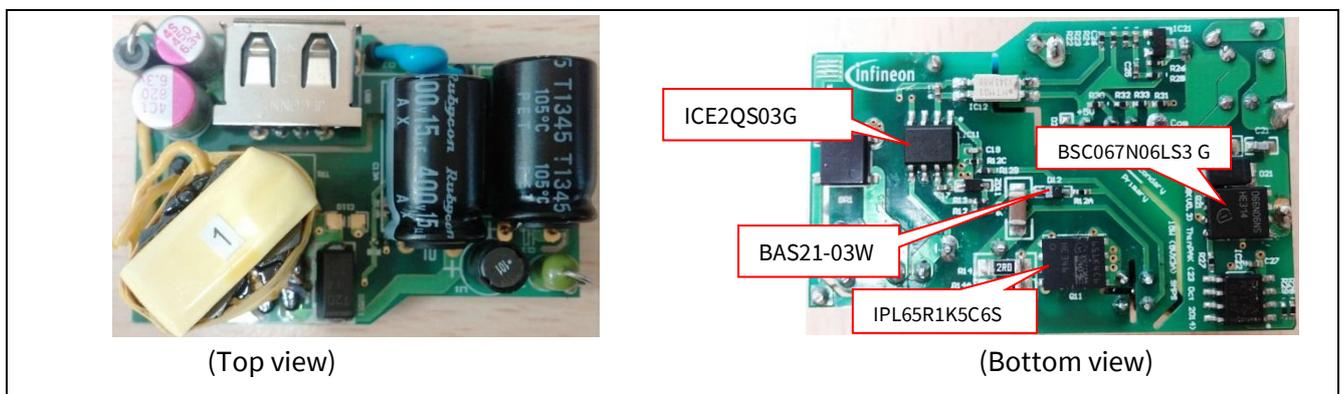
Figure 2 REF-15W\_C61K5-THINPAK ADAPTER [Top & Bottom View]
