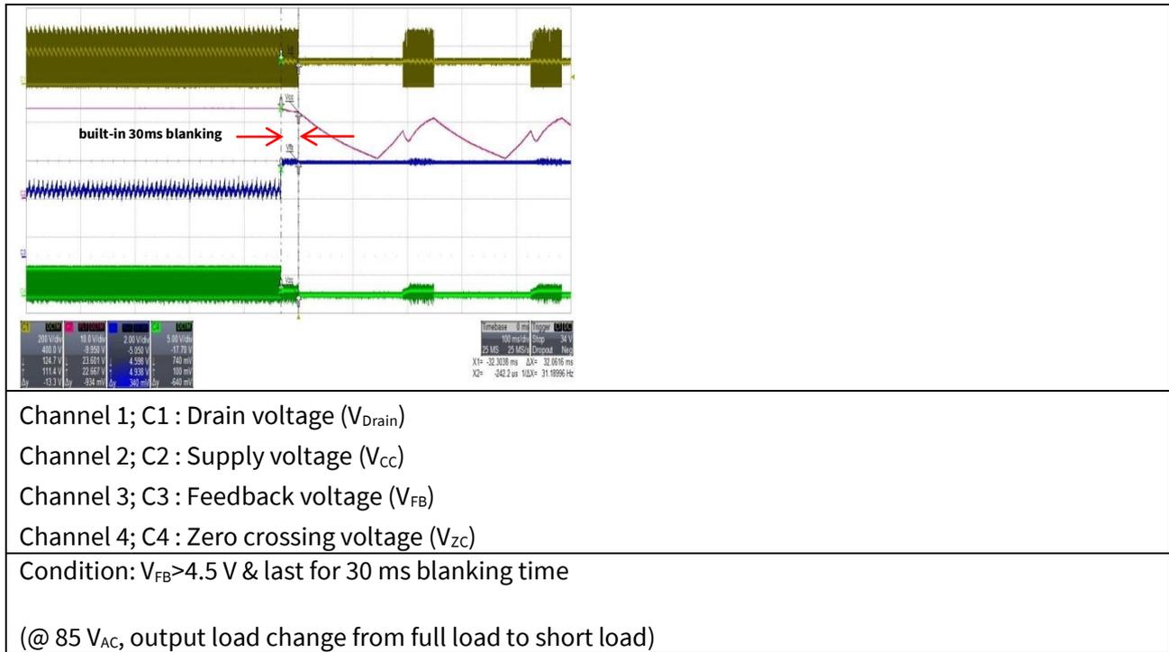
Figure 28 Over load protection
