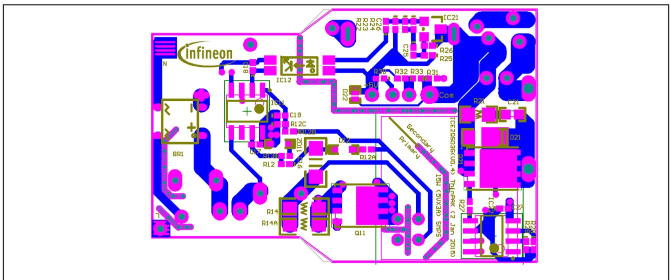
Figure 5 Bottom side copper and component legend
