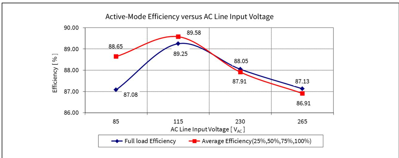
**Figure 7 Efficiency vs AC line input voltage**
