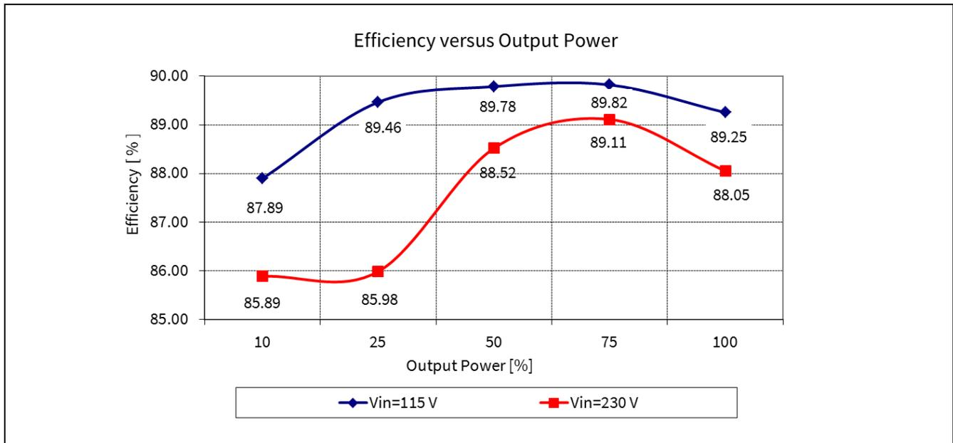
Figure 8 Efficiency vs output power @ 115 V<sub>AC</sub> and 230 V<sub>AC</sub> line
