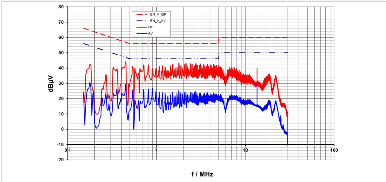
Figure 13 Conducted emissions(Line) at 115 V<sub>AC</sub> and maximum Load
