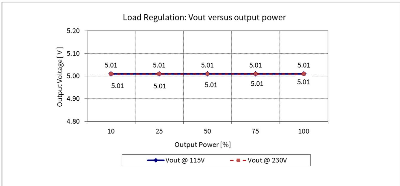
Figure 11 Load regulation  $V_{out}$  vs output power
