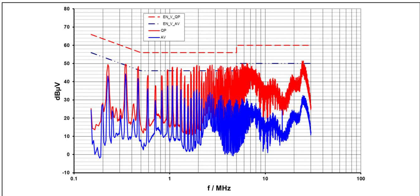
Figure 16 Conducted emissions(Neutral) at 230 V<sub>AC</sub> and maximum Load
