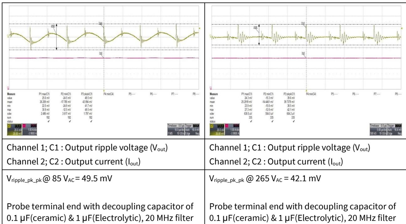
Figure 25 AC output ripple voltage at maximum load
