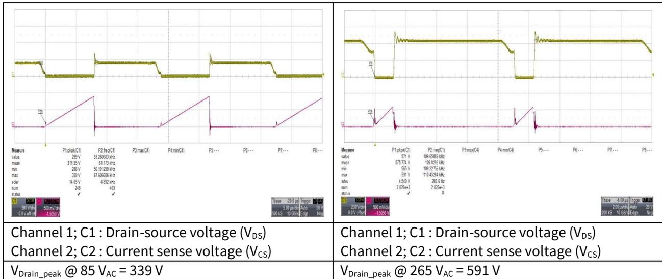
Figure 22 Drain & current sense voltage
