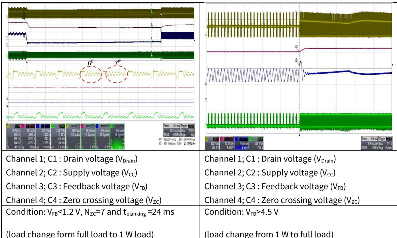
Figure 27 Active burst mode at 85  $V_{AC}$
