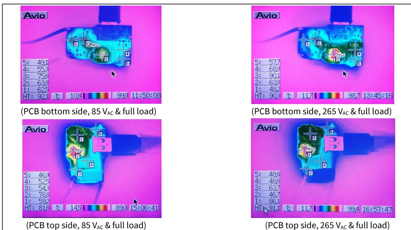
**Figure 17 Infrared thermal image of REF-15W\_C61K5-THINPAK ADAPTER**
