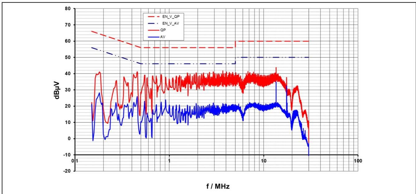
Figure 14 Conducted emissions(Neutral) at 115 V<sub>AC</sub> and maximum Load
