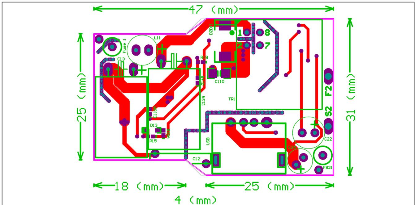
Figure 4 Top side copper and component legend
