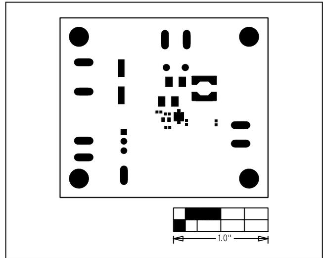
Figure 10. MAX17502F EV Kit PCB Layout—Top Solder Mask
