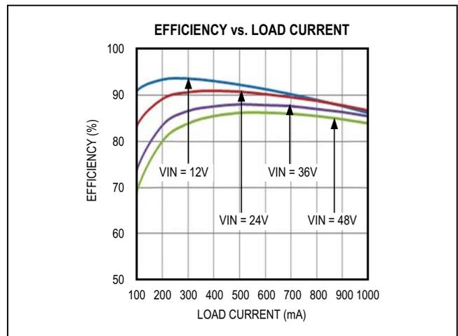
Figure 2. MAX17502F Efficiency
