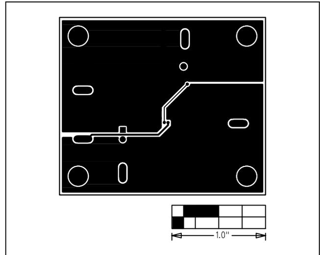
Figure 9. MAX17502F EV Kit PCB Layout—Solder Side
