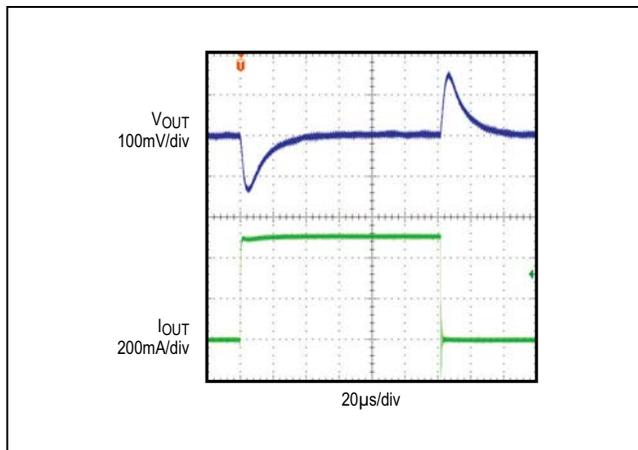
Figure 4. MAX17502F No Load to 500mA Load Transient
