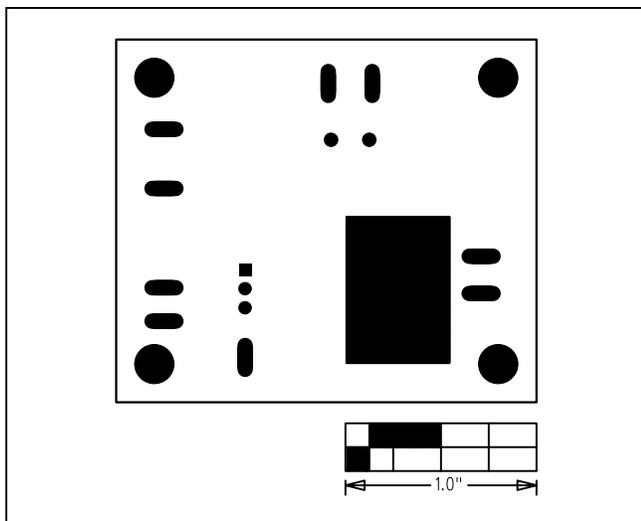
Figure 11. MAX17502F EV Kit PCB Layout—Bottom Solder Mask
