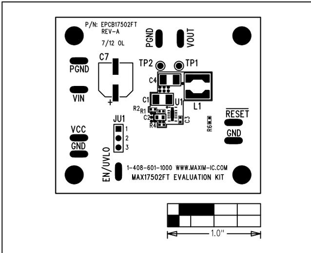
Figure 7. MAX17502F EV Kit Component Placement Guide—Component Side
