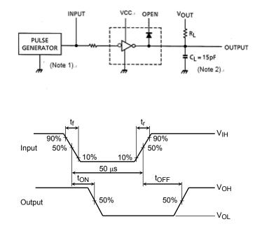
Note1: Pulse width 50  $\mu$ s, Duty cycle 10 % Output impedance 50  $\Omega$ , tr ≤ 5 ns, tf ≤ 10 ns, VIH = 5.0 V
