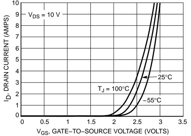
Figure 2. Transfer Characteristics
