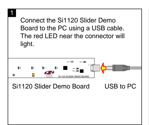
Wave your hand above the board. The visible blue LEDs will light according to the side-to-side position of your hand above the board. When a pause or swipe gesture is recognized, the LEDs will briefly flash a pattern to indicate the gesture and then return to indicating the position. Refer to the Si1120 Infrared Slider Demo User's Guide for more details.
