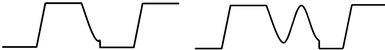
Figure 64. Full-load Operation – Quasi-resonant Mode in low line (left), turn on at valley 2 when in high line (right)
