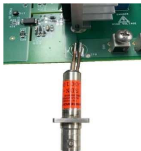
Figure 15. SDN-414-01 current viewing resistor (sold separately)
