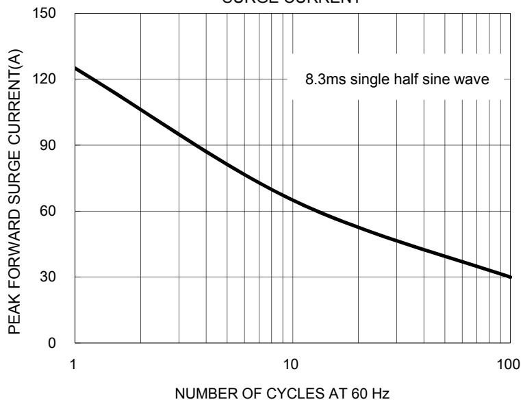
FIG. 3 MAXIMUM NON-REPETITIVE FORWARD SURGE CURRENT
