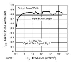
Fig. 2 - Output Pulse Width vs. Irradiance
