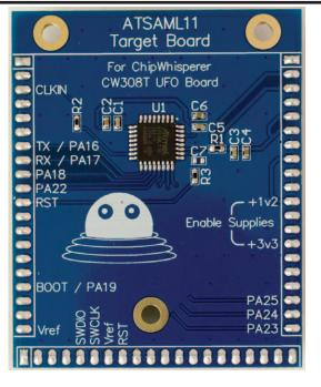
The SAML11 board features the ATSAML11 from Microchip. This device has a Cortex-M23 core, which features many advanced security features including TrustZone-M.
