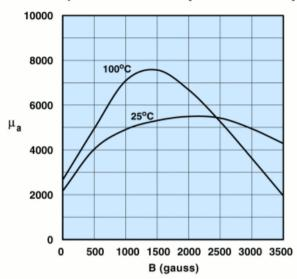
Measured on an 18/10/6mm toroid at 10kHz.
