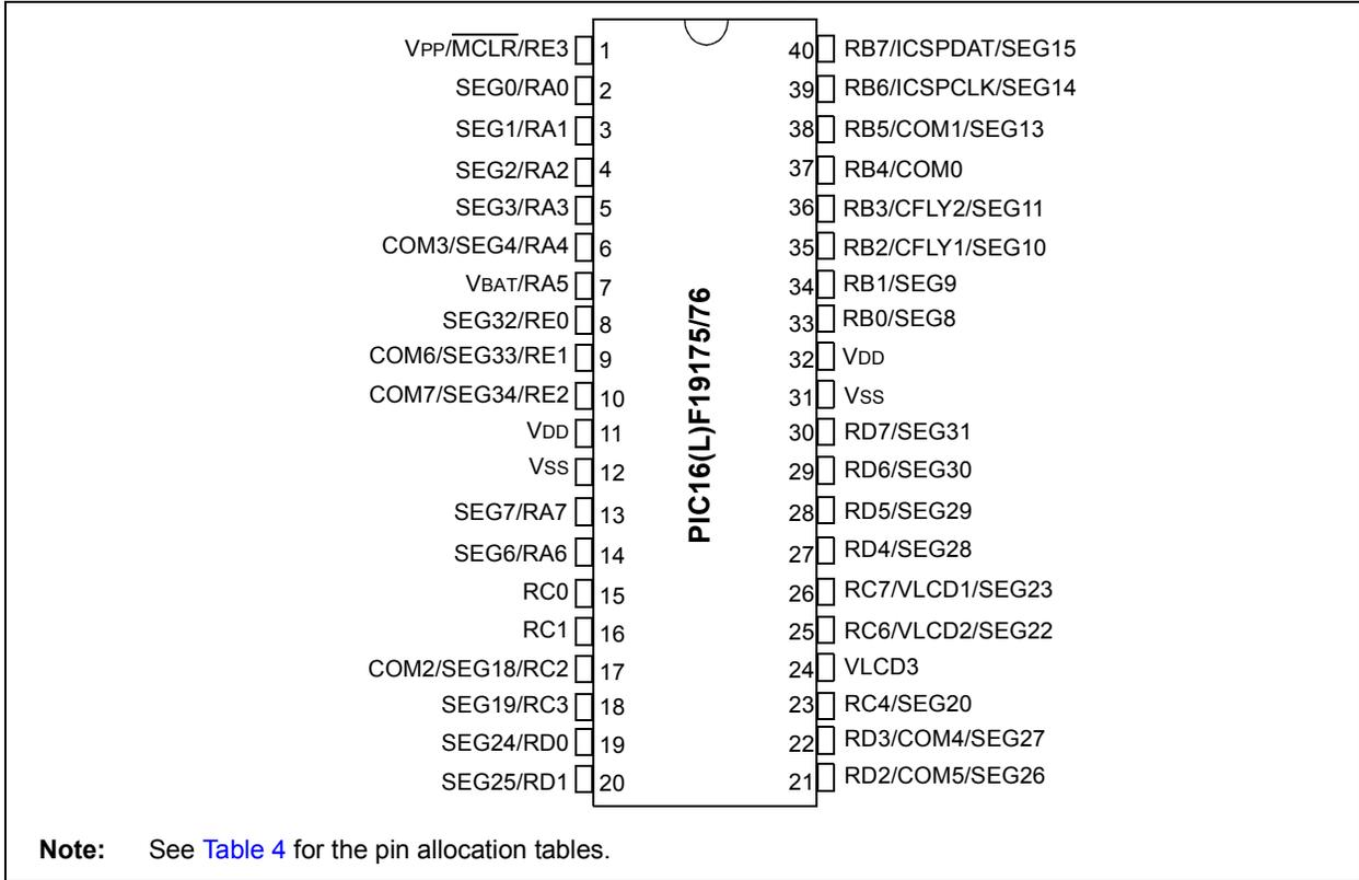
**FIGURE 4: 40-PIN UQFN (5X5X0,5) PIN DIAGRAM FOR PIC16(L)F19175/76**
