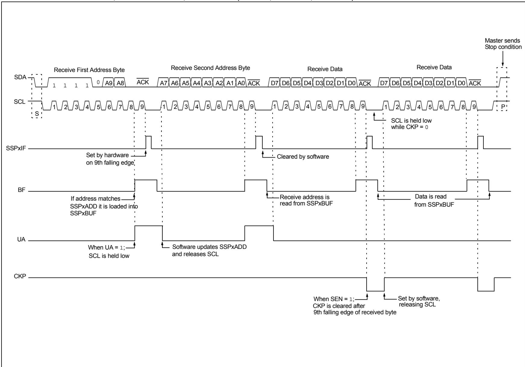
**FIGURE 33-21: I<sup>2</sup>C SLAVE, 10-BIT ADDRESS, RECEPTION (SEN = 0, AHEN = 1, DHEN = 0)**
