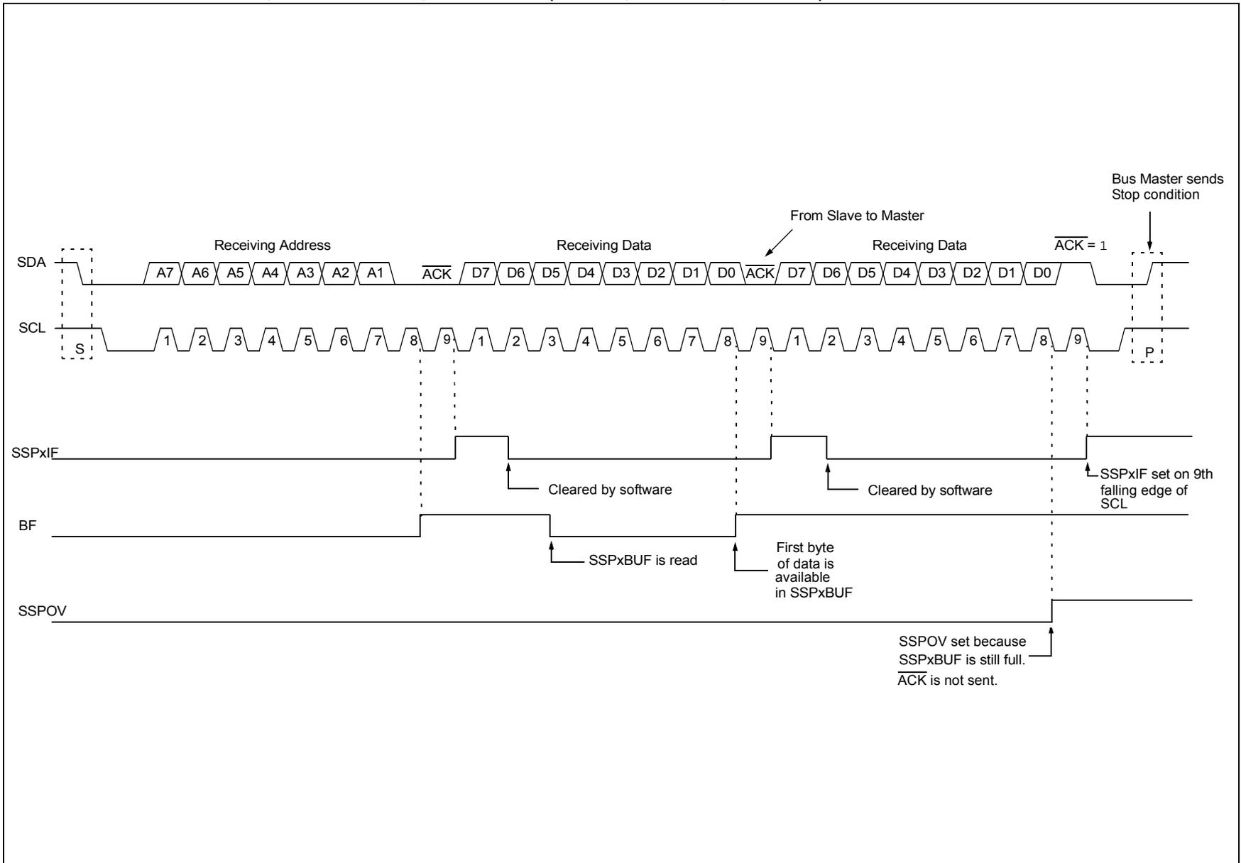
FIGURE 33-15: I<sup>2</sup>C SLAVE, 7-BIT ADDRESS, RECEPTION (SEN = 1, AHEN = 0, DHEN = 0)
