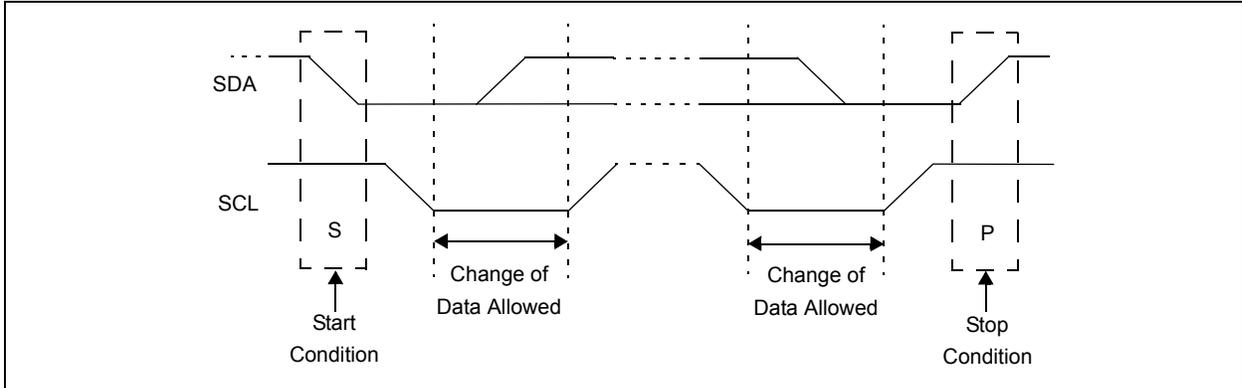
**FIGURE 33-13: I<sup>2</sup>C RESTART CONDITION**
