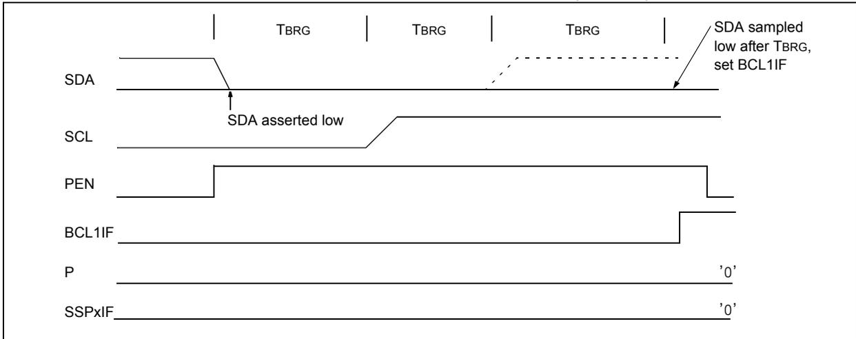
**FIGURE 33-39: BUS COLLISION DURING A STOP CONDITION (CASE 2)**
