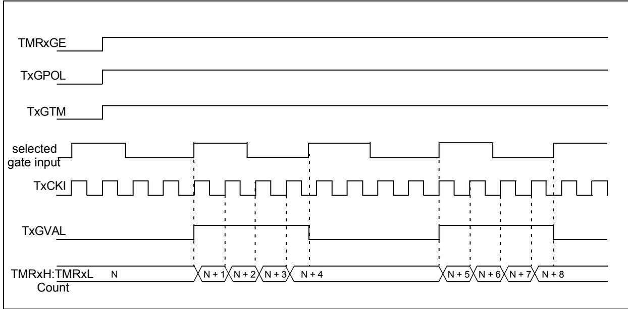
**FIGURE 26-5: TIMER1 GATE SINGLE-PULSE MODE**
