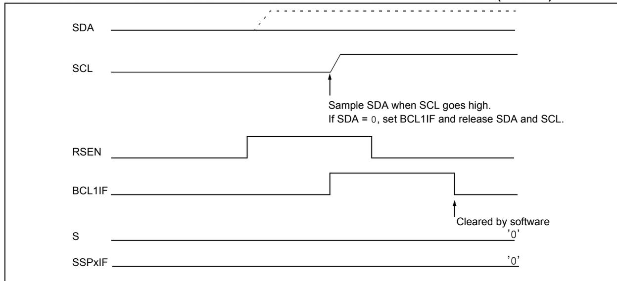
**FIGURE 33-37: BUS COLLISION DURING REPEATED START CONDITION (CASE 2)**
