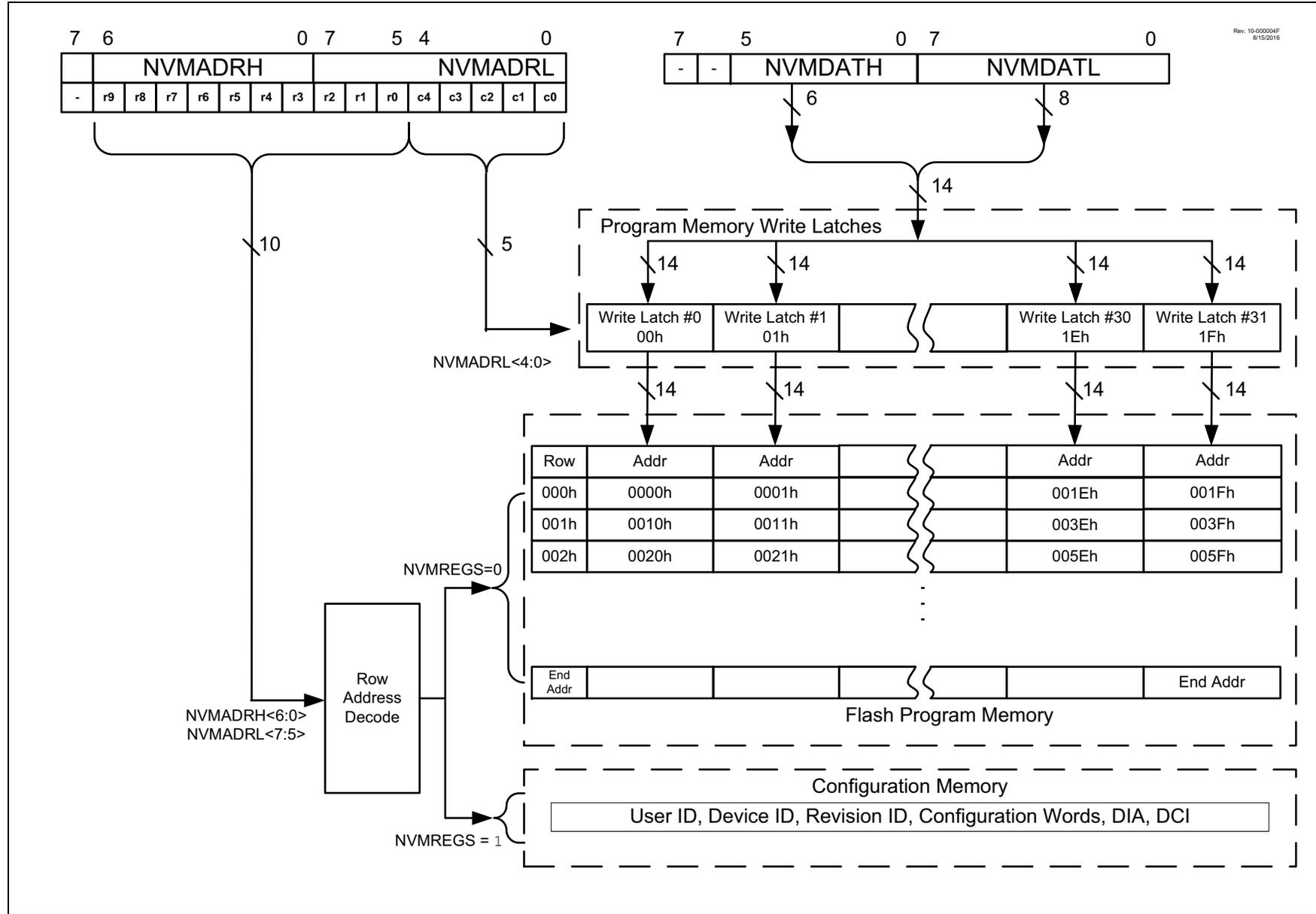
**FIGURE 13-5: PROGRAM FLASH MEMORY (PFM) WRITE FLOWCHART**
