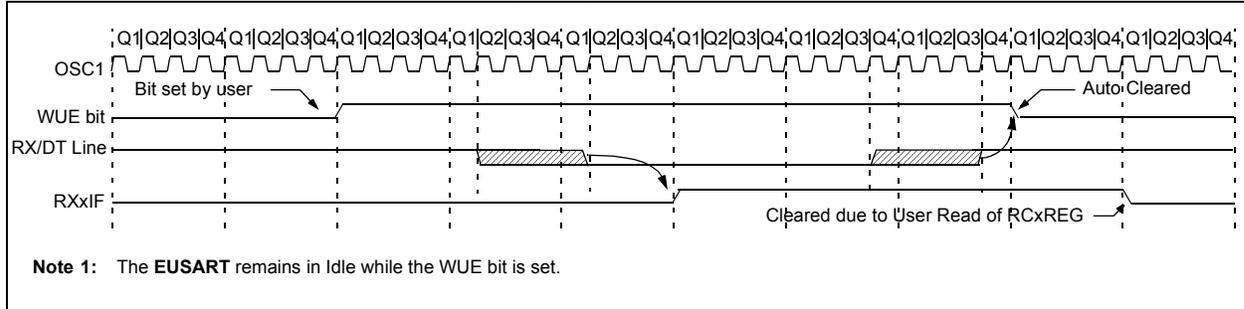
**FIGURE 34-8: AUTO-WAKE-UP BIT (WUE) TIMINGS DURING SLEEP**
