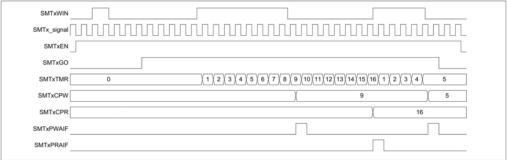
**FIGURE 28-22: WINDOWED COUNTER MODE SINGLE ACQUISITION TIMING DIAGRAM**
