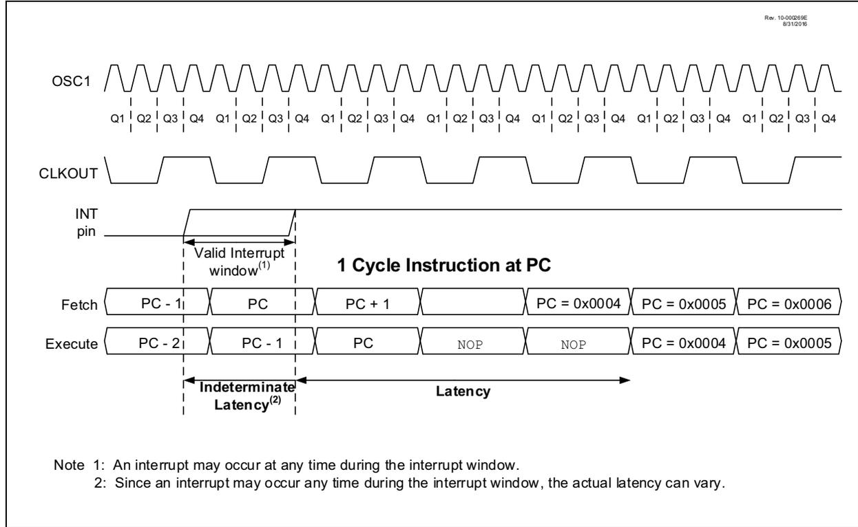
**FIGURE 10-3: INT PIN INTERRUPT TIMING**
