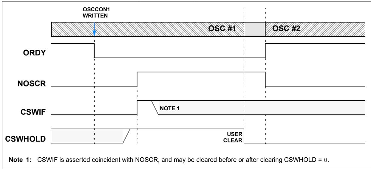
**FIGURE 9-6: CLOCK SWITCH ABANDONED**
