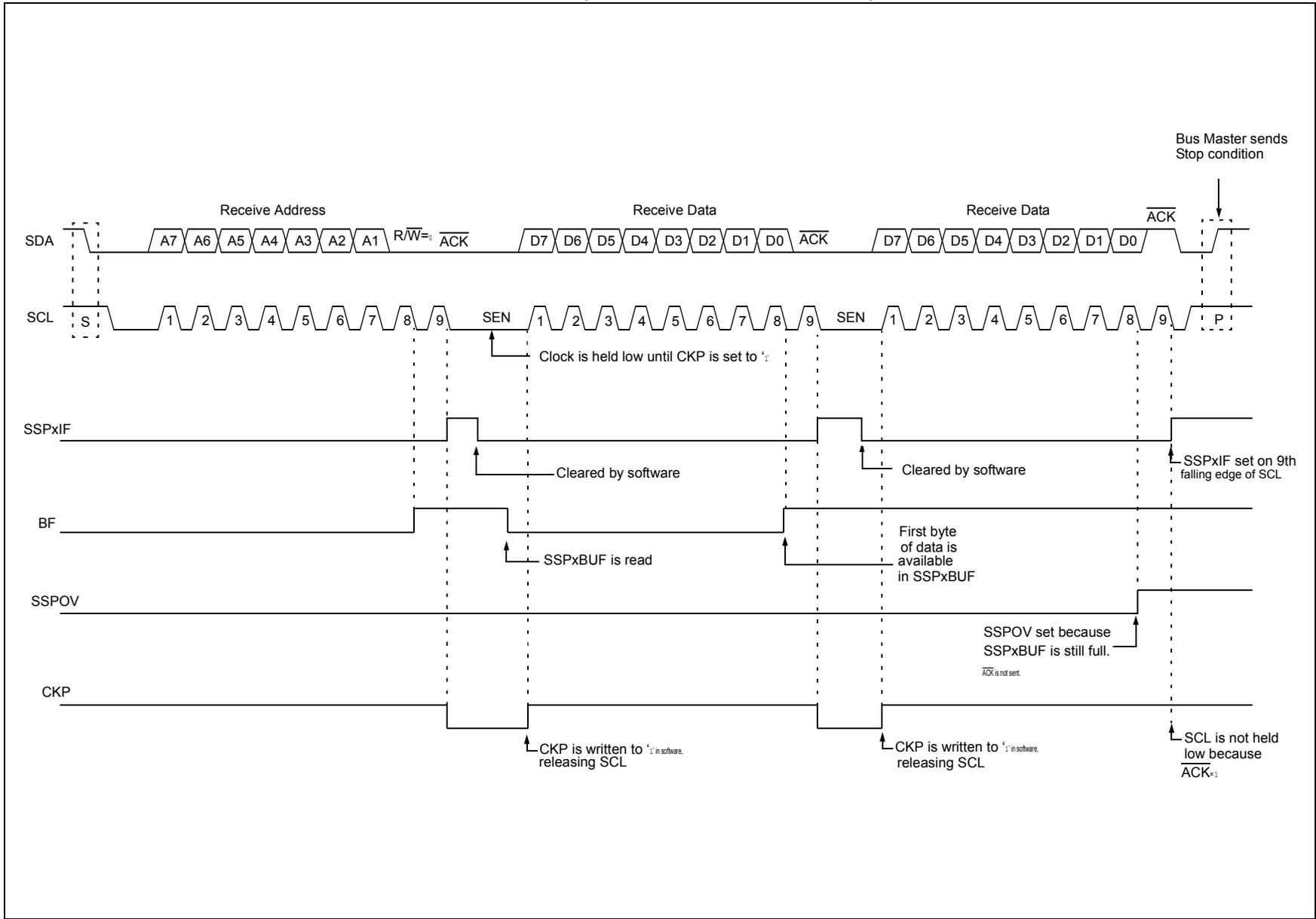
**FIGURE 33-16: I<sup>2</sup>C SLAVE, 7-BIT ADDRESS, RECEPTION (SEN = 0, AHEN = 1, DHEN = 1)**
