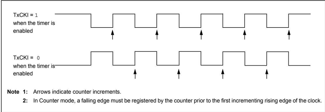
**FIGURE 26-3: TIMER1 GATE ENABLE MODE**
