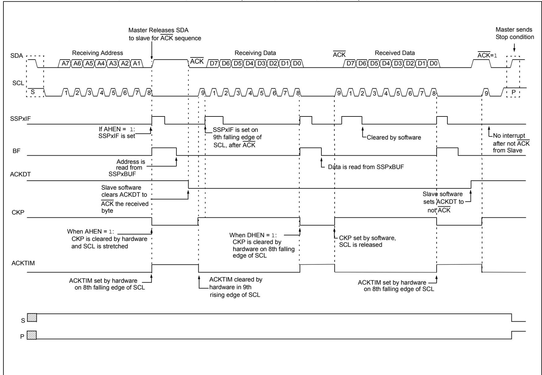
**FIGURE 33-17: I<sup>2</sup>C SLAVE, 7-BIT ADDRESS, RECEPTION (SEN = 1, AHEN = 1, DHEN = 1)**
