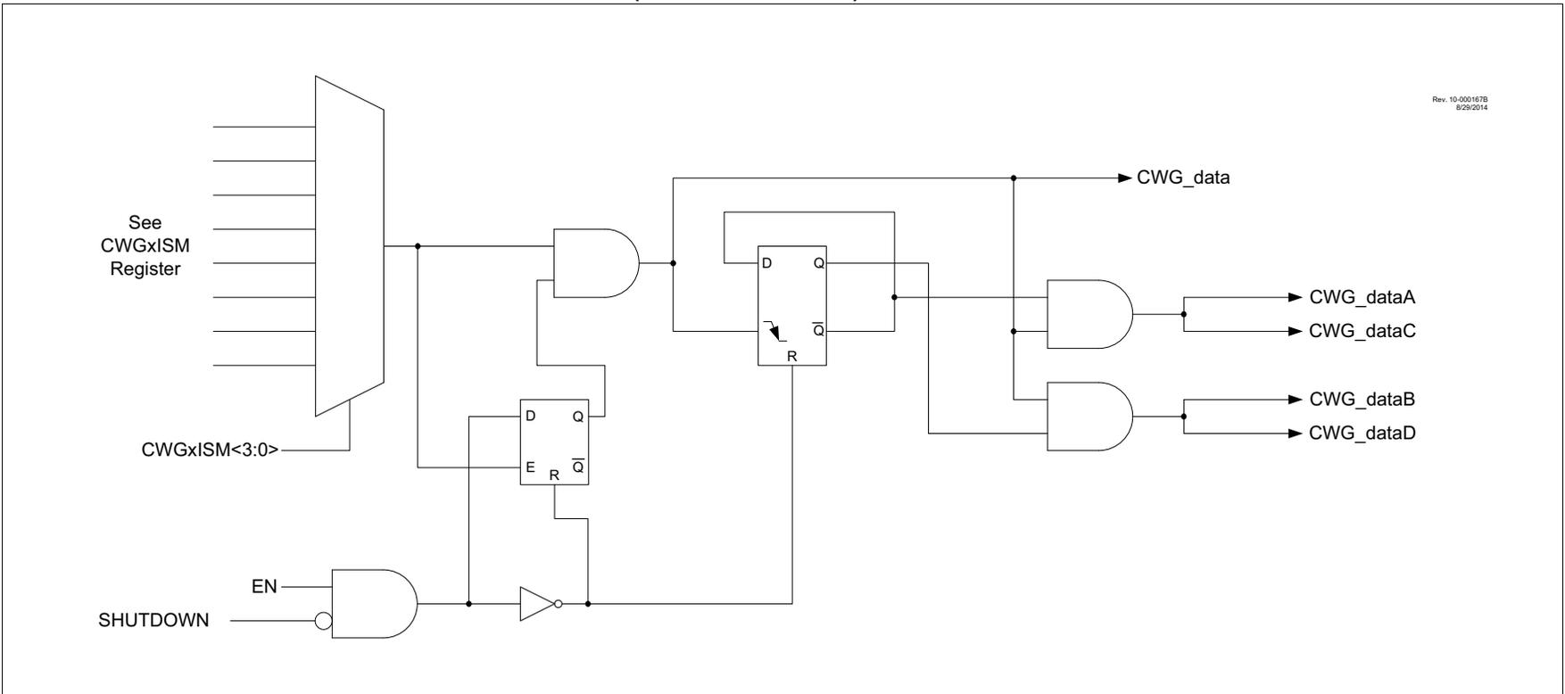
FIGURE 31-3: SIMPLIFIED CWG BLOCK DIAGRAM (FORWARD AND REVERSE FULL-BRIDGE MODES)
