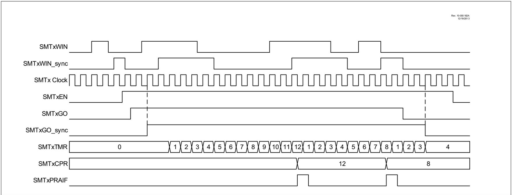
FIGURE 28-11: WINDOWED MEASURE MODE SINGLE ACQUISITION TIMING DIAGRAM
