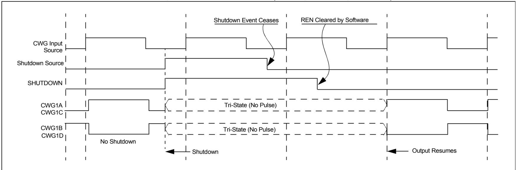
**FIGURE 31-14: SHUTDOWN FUNCTIONALITY, AUTO-RESTART ENABLED (REN = 1, LSAC = 01, LSBD = 01)**
