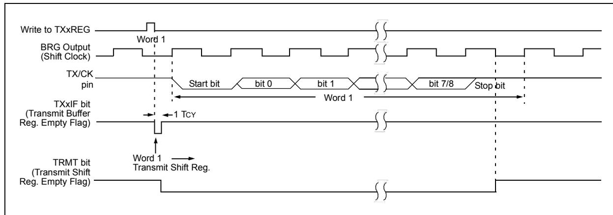
**FIGURE 34-4: ASYNCHRONOUS TRANSMISSION (BACK-TO-BACK)**
