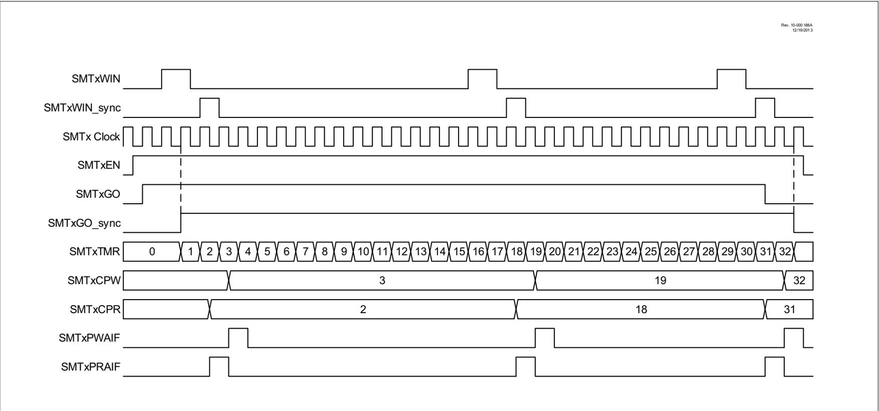
**FIGURE 28-17: CAPTURE MODE SINGLE ACQUISITION TIMING DIAGRAM**
