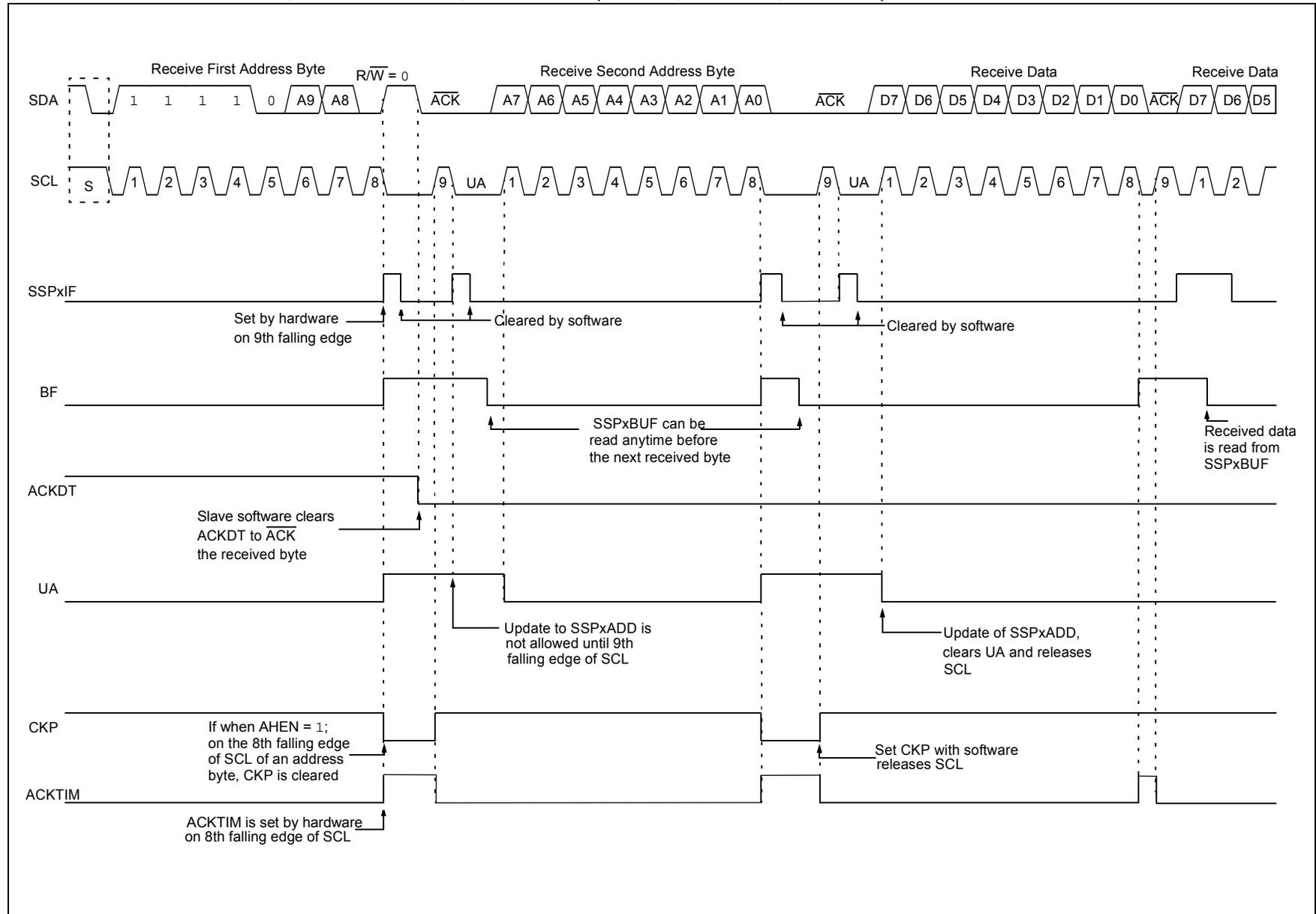
**FIGURE 33-22: I<sup>2</sup>C SLAVE, 10-BIT ADDRESS, TRANSMISSION (SEN = 0, AHEN = 0, DHEN = 0)**
