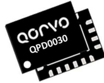
20 Pin 3 x 4 mm QFN Package
