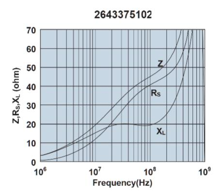
Impedance, reactance, and resistance vs. frequency.
