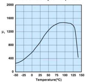
Measured on a 17/10/6mm toroid at 100kHz.
