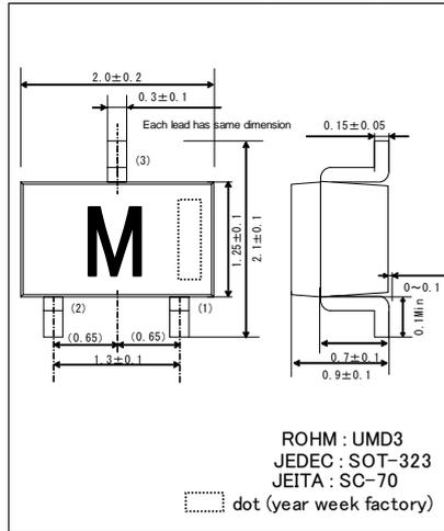
●Lead size figure (Unit : mm)
