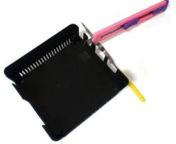
**Step 3 (optional)**- **Connect the Wi-Fi cable**: plug the cable in the  $\mu$ FL IPEX connector and lead it through the open hole to the other side
