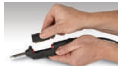
Collection chamber replacement
