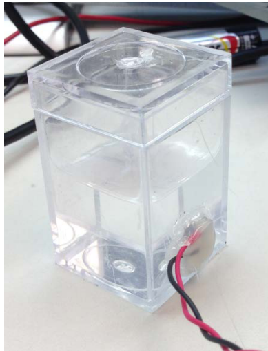
Figure 2. Water Container with 1-MHz Transducer
