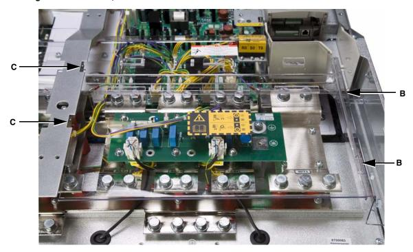
Figure 20: Left Terminal Shield, Frame Size 15
